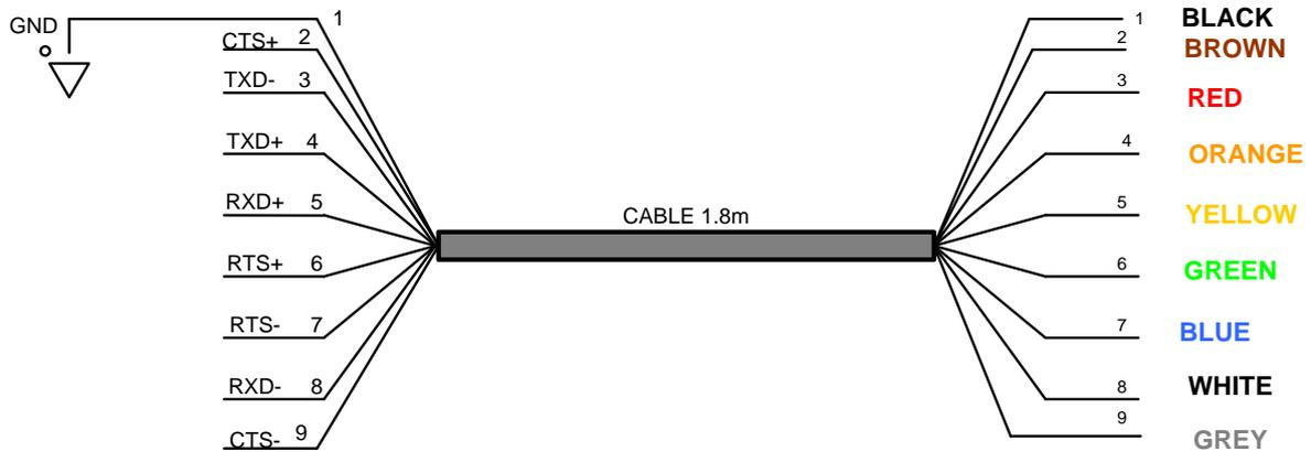
**Figure 5.1 USB-RS422-WE Connections**
