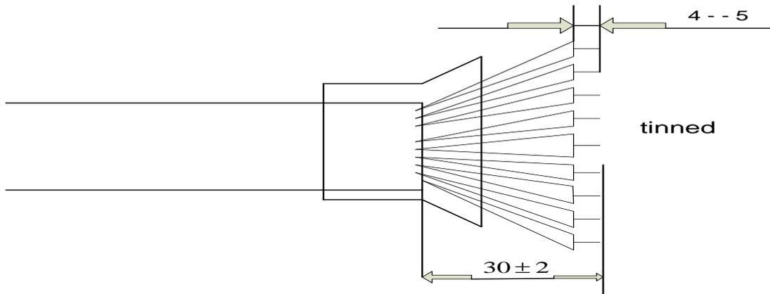
**Figure 5.2 USB-RS422-WE Mechanical Details (dimensions in mm)**
