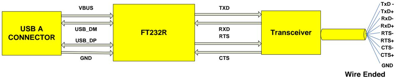
**Figure 6.1 Block diagram of PCB Used in the USB to RS422 Serial Converter Cable**
