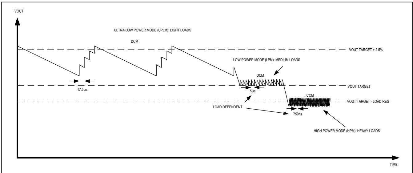
Figure 4. ULPM, LPM, and HPM Waveforms (Part 1).
