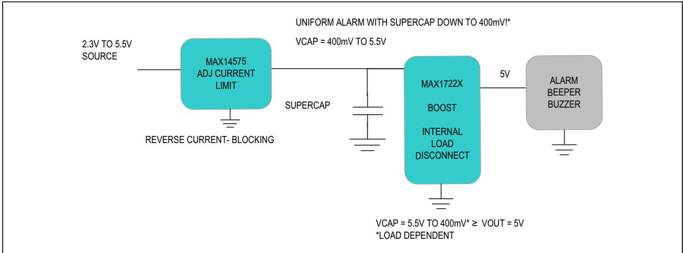
Figure 11. MAX1722x/MAX14575 Solution for Alarm Beeper Buzzers.
