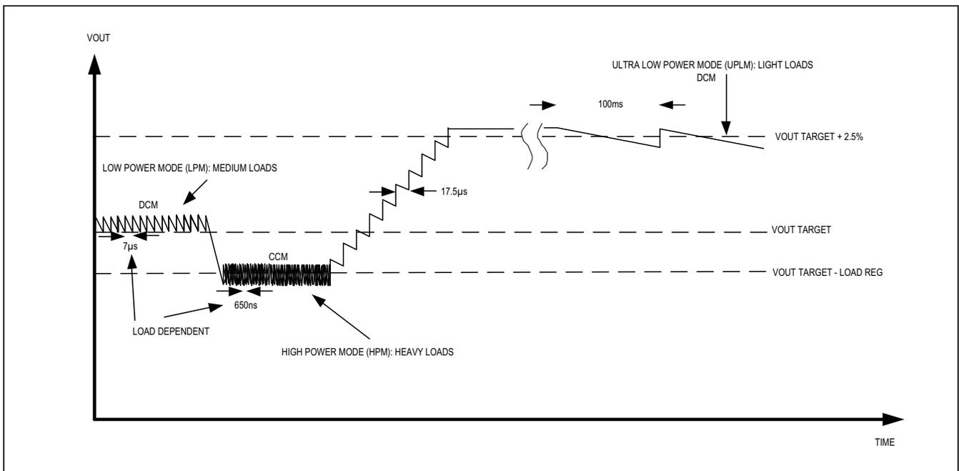
Figure 5. ULPM, LPM, and HPM Waveforms (Part 2).
