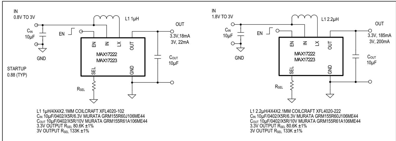
Highest Efficiency Solution—4 x 4mm Inductor—MAX17222/MAX17223 500mA I<sub>LIM</sub> (Part 2)
