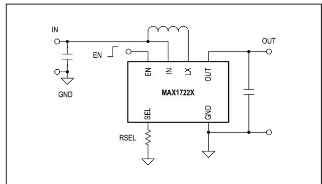
Figure 6. Single RSEL Resistor Sets the Output Voltage.
