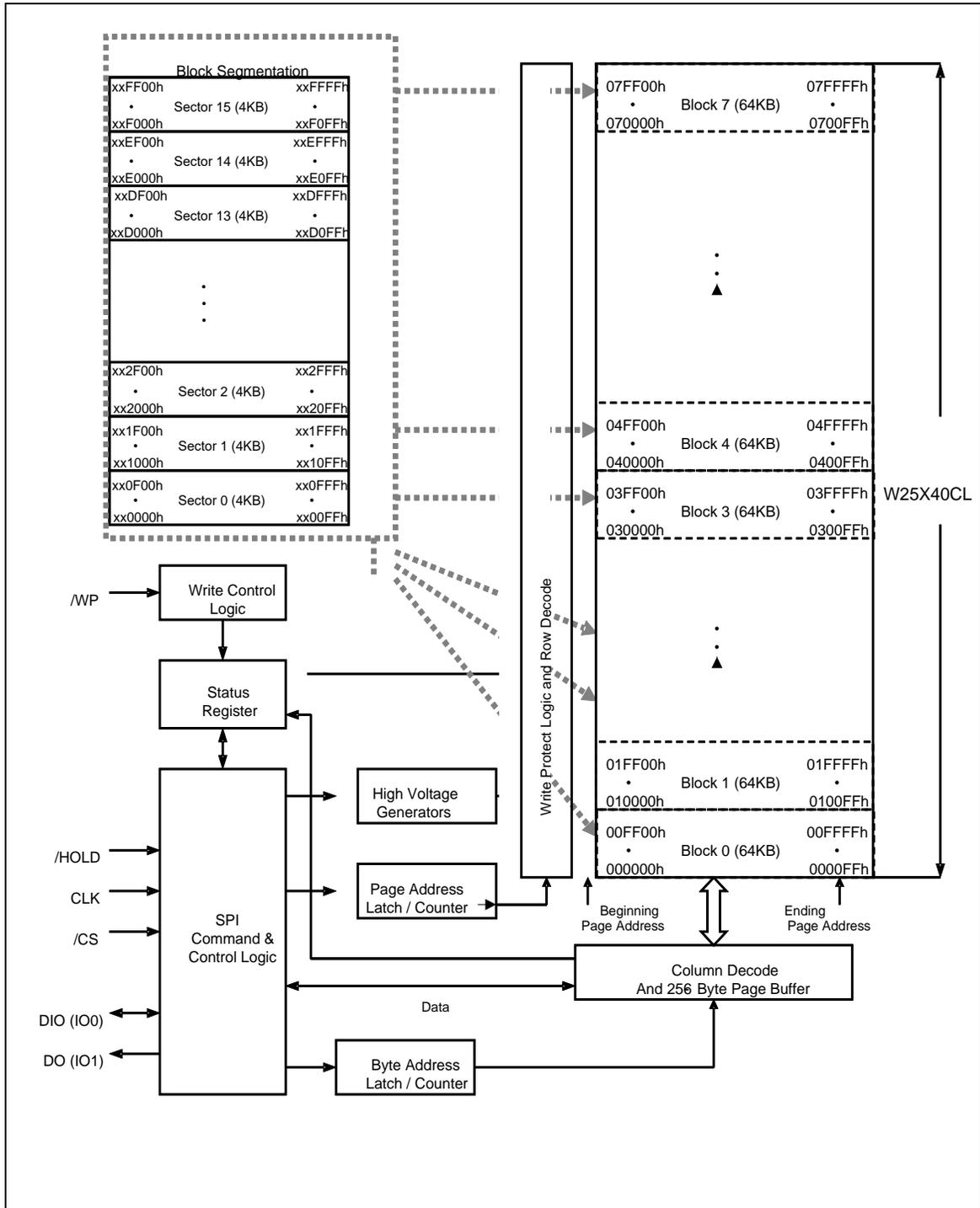
Figure 2. W25X40CL Serial Flash Memory Block Diagram
