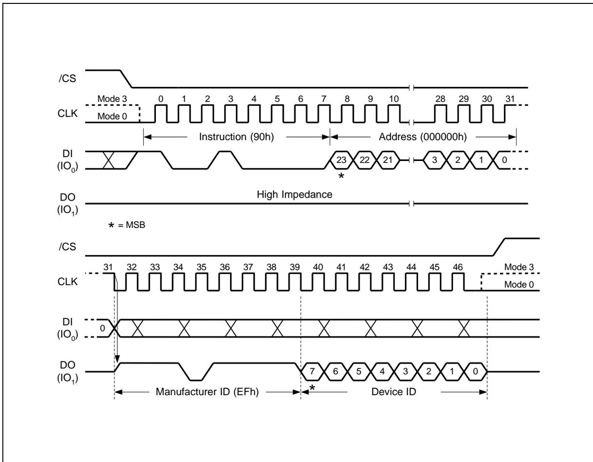
Figure 22. Read Manufacturer / Device ID Diagram
