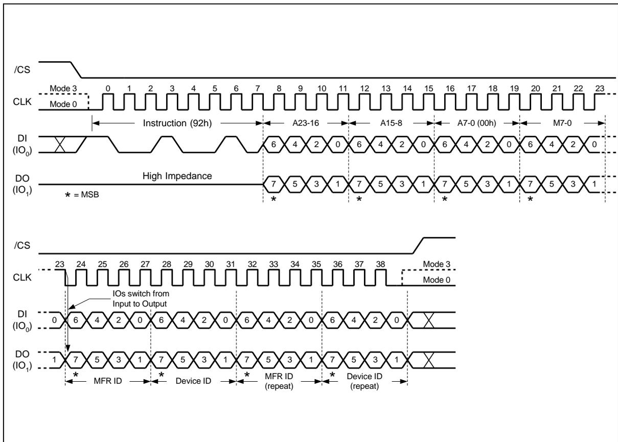
Figure 23. Read Manufacturer / Device ID Dual I/O Diagram
