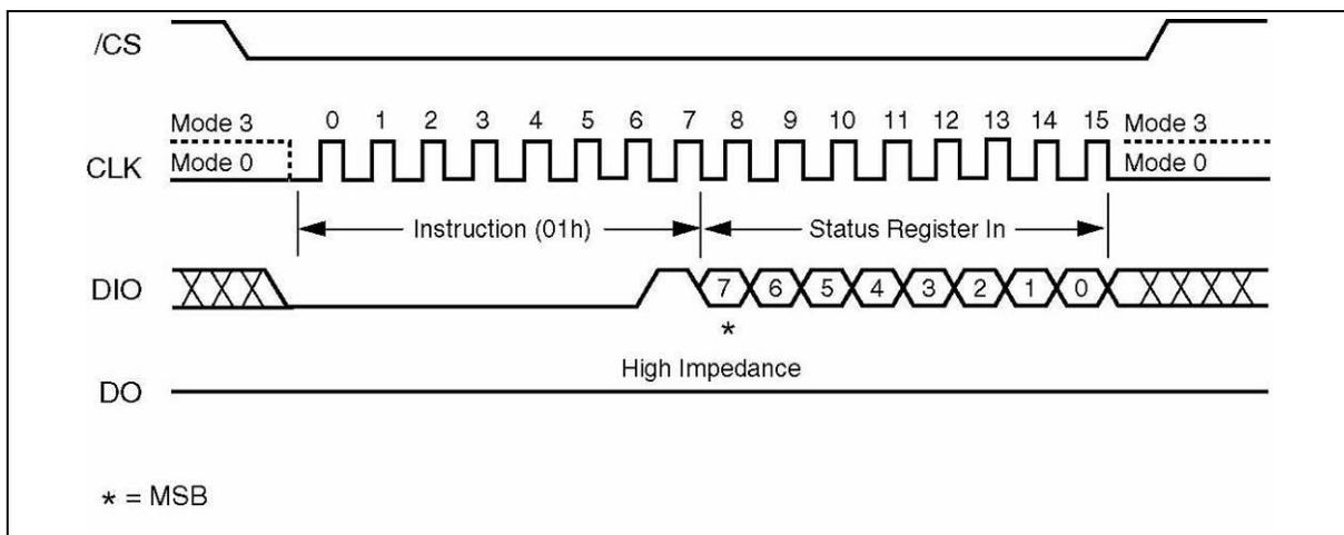
Figure 8. Write Status Register Instruction Sequence Diagram
