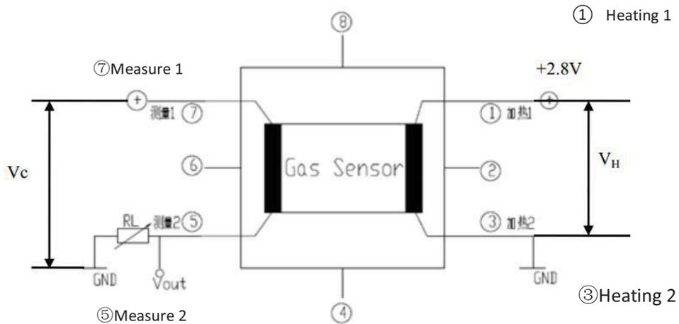
Fig2. GM-302B test circuit
