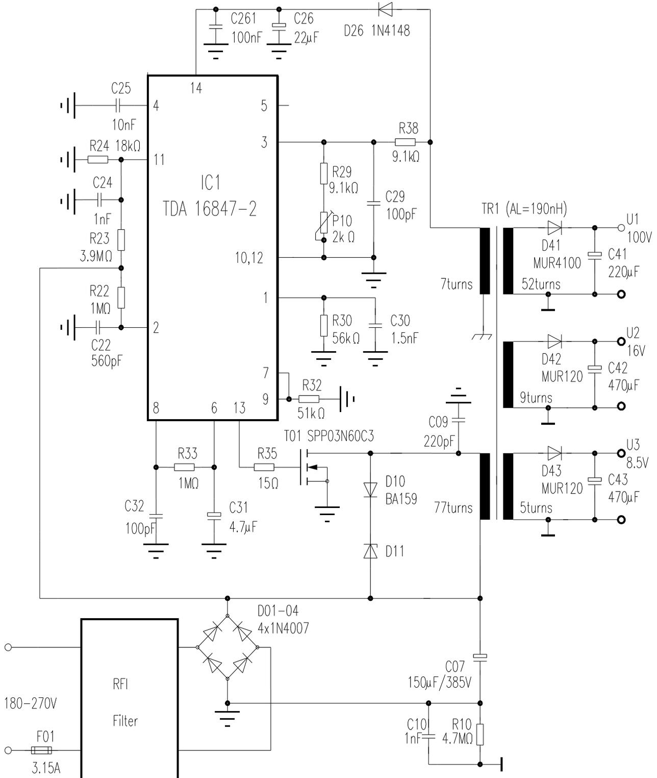
**Figure 17**    **Circuit Diagram for Application with Temporary High Power Circuit**
