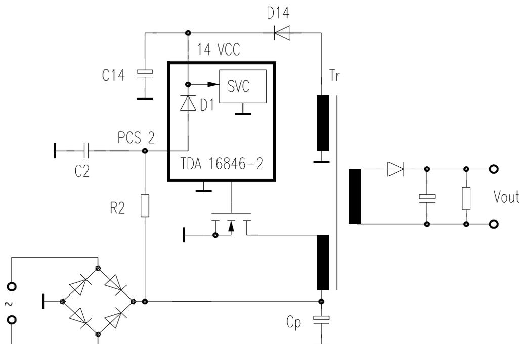
**Figure 4 Startup Circuit**
