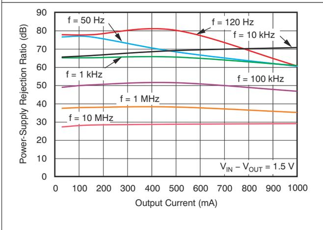
Figure 6-11. Power-Supply Rejection Ratio vs Output Current
