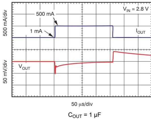
Figure 6-15. Load Transient Response 1 mA to 500 mA
