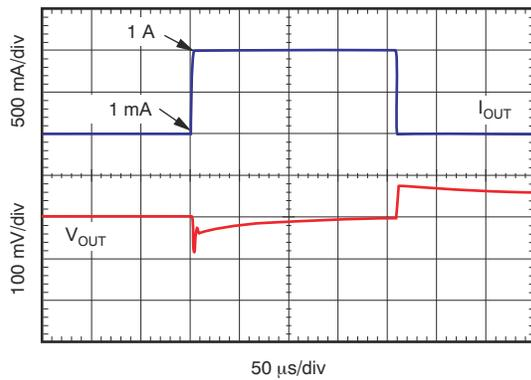
**Figure 6-19. Load Transient Response 1 mA to 1 A**
