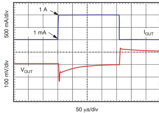
**Figure 6-20. Load Transient Response 1 mA to 1 A**
