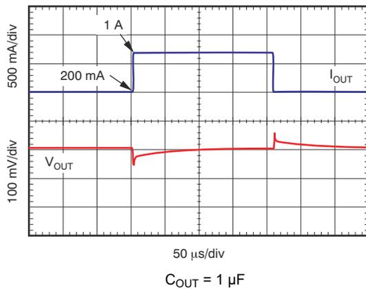
Figure 6-17. Load Transient Response 200 mA to 1 A
