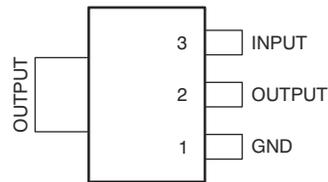
**Figure 5-1. DCY Package, 4 Pins (SOT-223) (Top View)**
