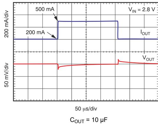
Figure 6-14. Load Transient Response 200 mA to 500 mA
