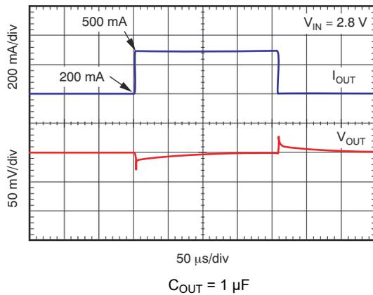
Figure 6-13. Load Transient Response 200 mA to 500 mA
