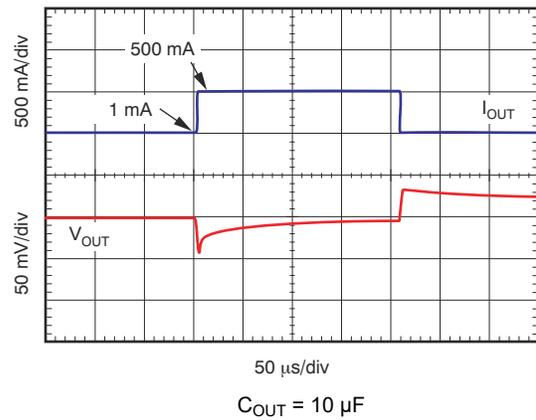
Figure 6-16. Load Transient Response 1 mA to 500 mA
