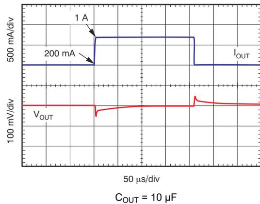
Figure 6-18. Load Transient Response 200 mA to 1 A
