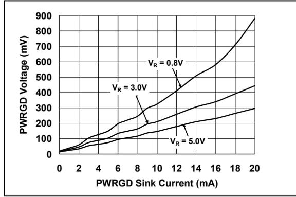
**FIGURE 2-33:** Power Good Pulldown Voltage Vs Load.
