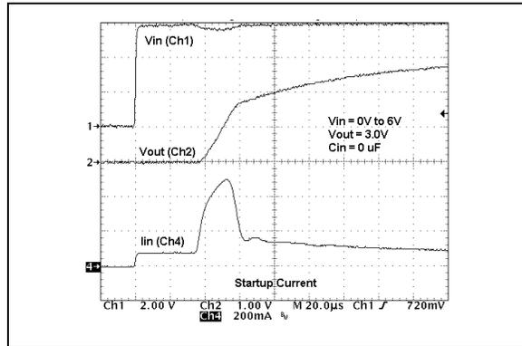
**FIGURE 2-34:** Startup Current.
