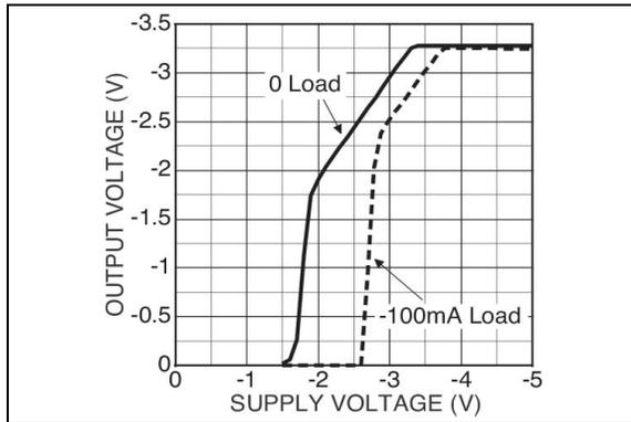
**FIGURE 2-1:** Dropout Characteristics.
