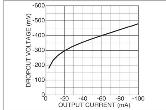
**FIGURE 2-10:** Dropout vs. Output Current.
