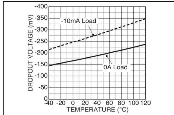
**FIGURE 2-11:** Dropout vs. Temperature.
