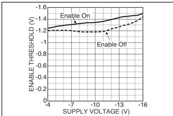
**FIGURE 2-9:** Negative Enable Threshold vs. Supply Voltage.
