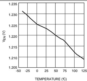
**Figure 3. Enable Threshold vs Temperature**
