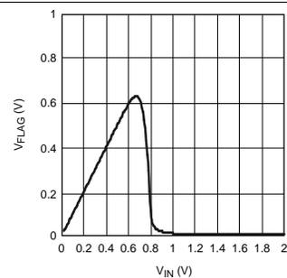
**Figure 6.  $V_{FLAG}$  vs  $V_{IN}$  (INV Low,  $R_{FLAG} = 100\text{ k}\Omega$ )**
