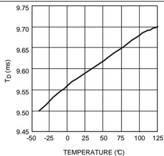
**Figure 5. Time Delay vs Temperature ( $C_{ADJ} = 10\text{ nF}$  Nominal)**
