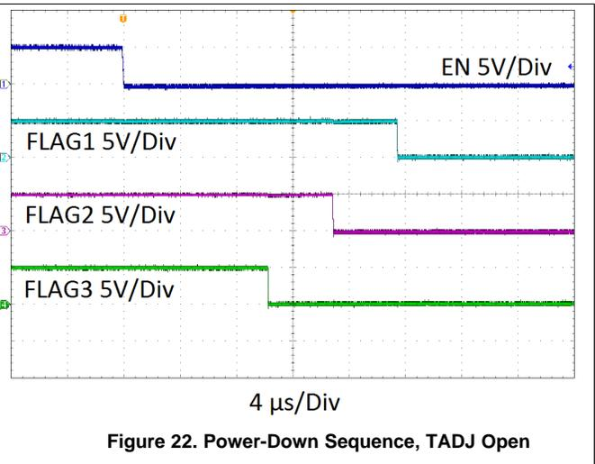
Figure 22. Power-Down Sequence, TADJ Open
