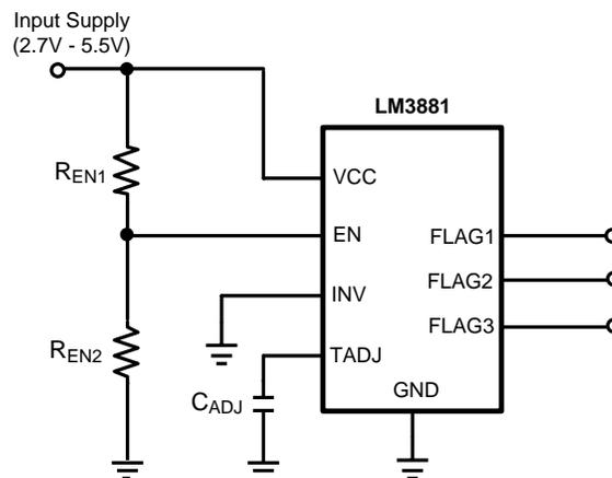
Figure 15. Enable Based On Input Supply Level
