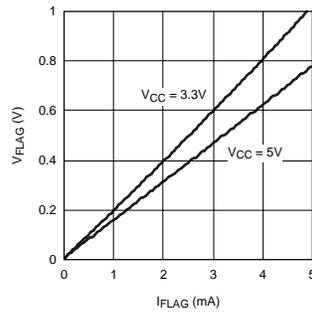
**Figure 7. FLAG Voltage vs Current**
