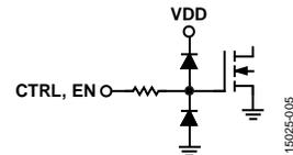
Figure 5. Digital Pins (CTRL and EN) Interface Schematic
