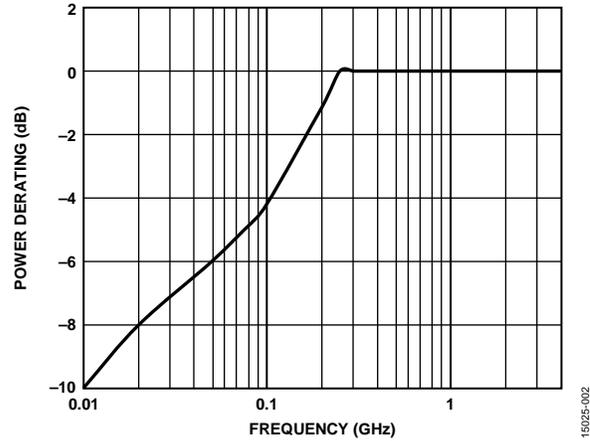
Figure 2. Power Derating at Frequencies Less Than 250 MHz
