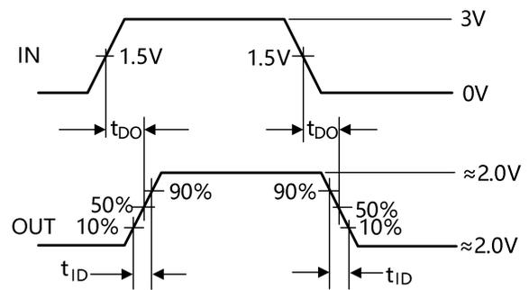
Figure 5. Driver Differential Output Delay and Transition Times
