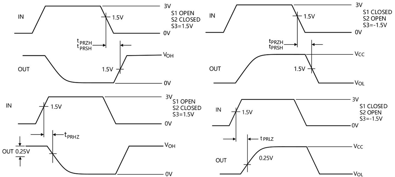
Figure 10. Driver Enable and Disable Times ( $T_{PZH}$ ,  $T_{PSH}$ ,  $T_{PHZ}$ )
