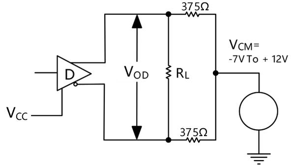
Figure 3. Driver  $V_{OD}$  with Varying Common-Mode Voltage
