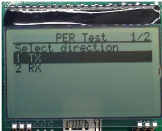
For the packet error rate test, set one of the boards up as the receiver (RX) and the other as the transmitter (TX).
