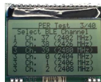
Then select the type of test you want to run. Packet mode is the Packet Error Rate test. CW is a continuous wave signal, either modulated or unmodulated.
