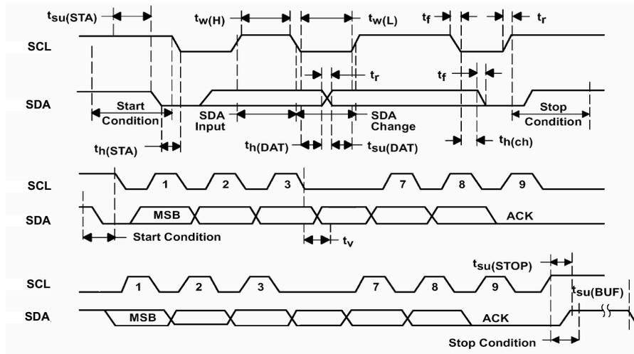
Figure 7-1. I<sup>2</sup>C Timing
