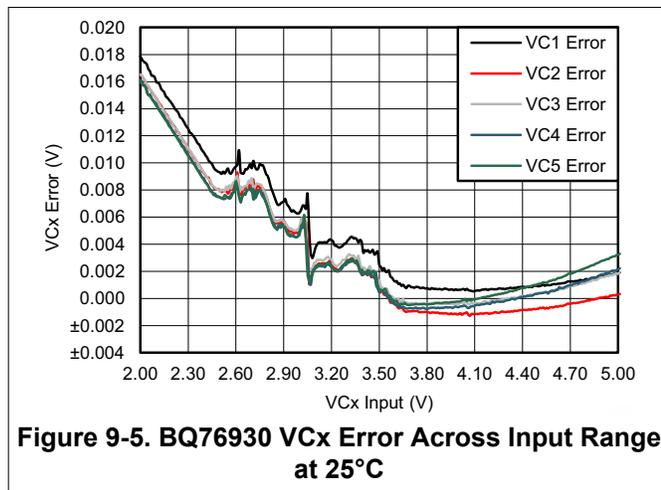
**Figure 9-5. BQ76930 VCx Error Across Input Range at 25°C**
