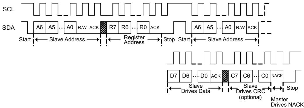
Figure 8-5. I<sup>2</sup>C Read Without Repeated Start
