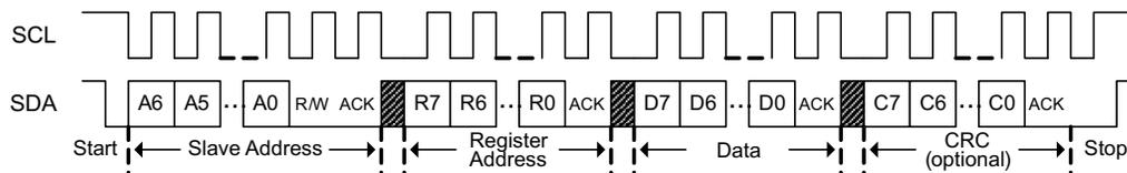
**Figure 8-3. I<sup>2</sup>C Write**
