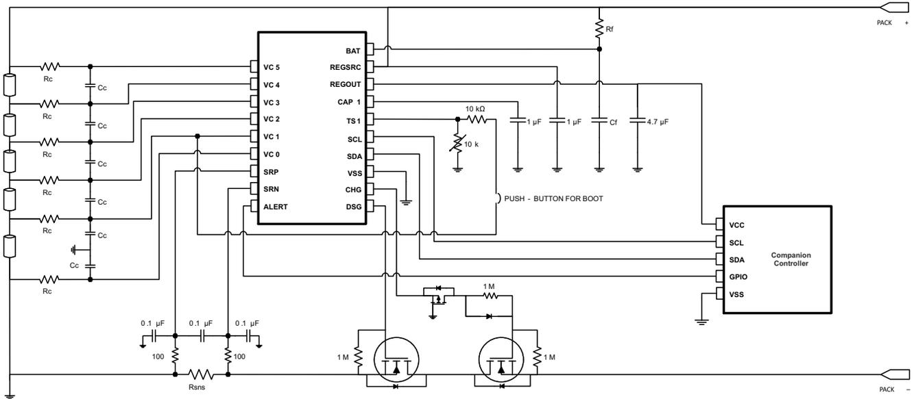
Figure 9-1. BQ76920 with BQ78350 Companion Controller IC
