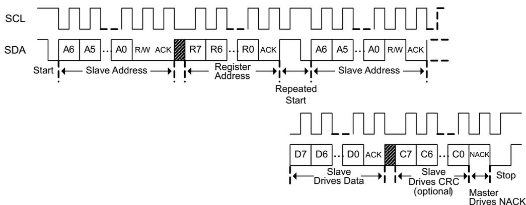
**Figure 8-4. I<sup>2</sup>C Read with Repeated Start**
