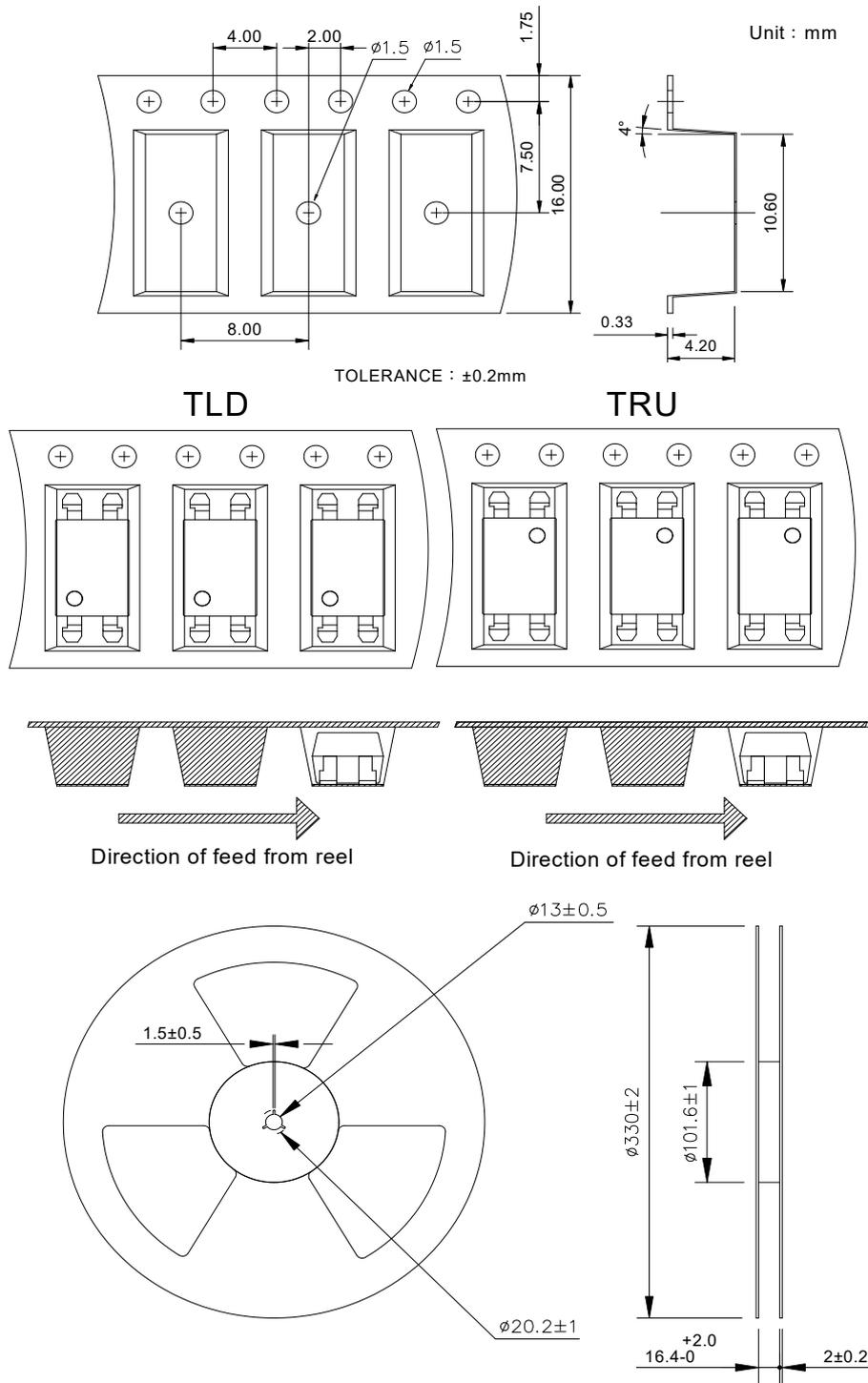
● 4-pin SOP Carrier Tape & Reel
