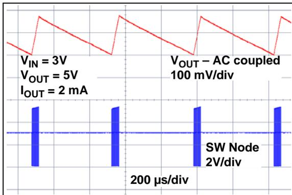
**FIGURE 4:** MCP16251 Output Voltage.
