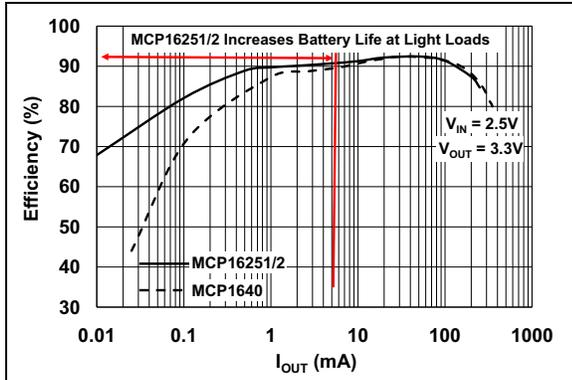
**FIGURE 3:** Efficiency vs. Output Current.
