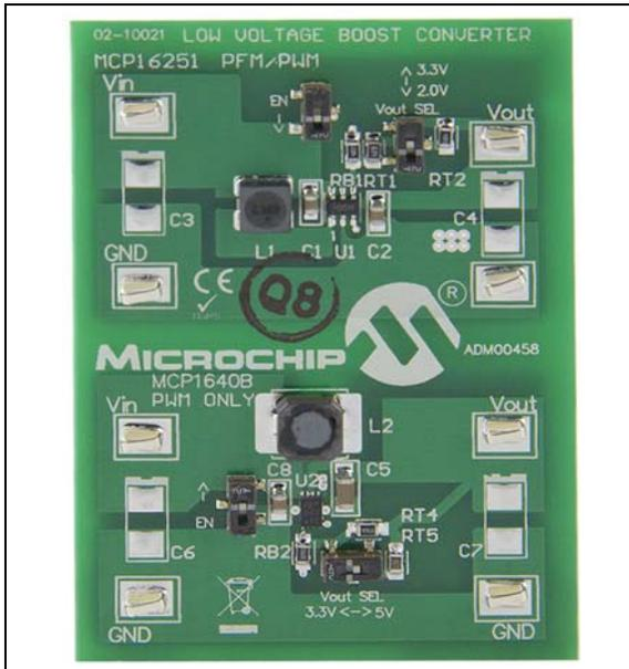
**FIGURE 6:** MCP16251 and MCP1640B Evaluation Board.
