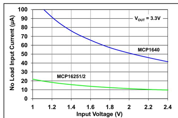
**FIGURE 2:** No Load Input Current.
