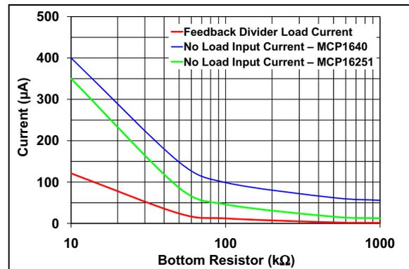
**FIGURE 1:** No Load Input Current ( $V_{IN} = 1.5V$ ,  $V_{OUT} = 3.3V$ ).
