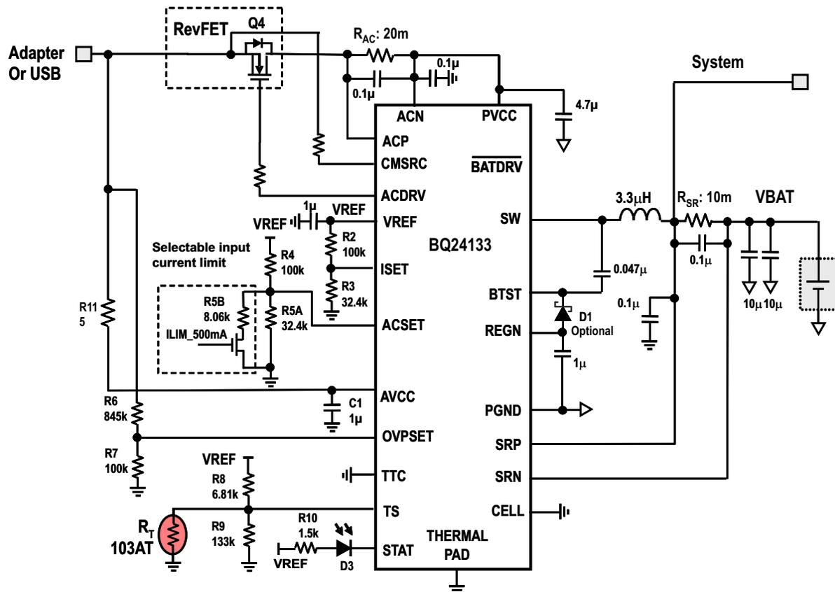
USB or adapter with input OVP 15 V, up to 2-A charge current, 0.2-A precharge current, 2-A adapter current or 500-mA USB current, 5 – 40°C TS, system connected before sense resistor
