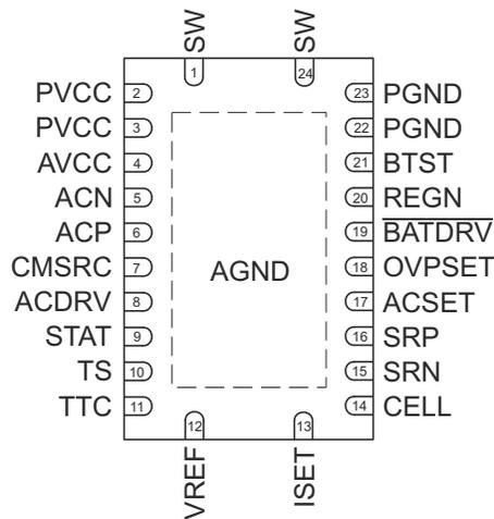
**Figure 7-1. RGY Package 24-Pin VQFN Top View**
