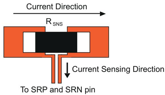
Figure 12-2. Sensing Resistor PCB Layout
