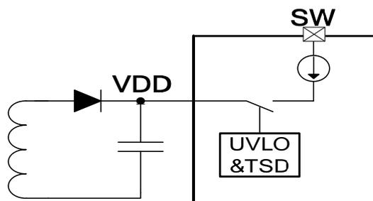
Fig 2. Startup circuit
