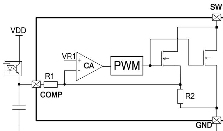
Fig 3. Feedback circuit
