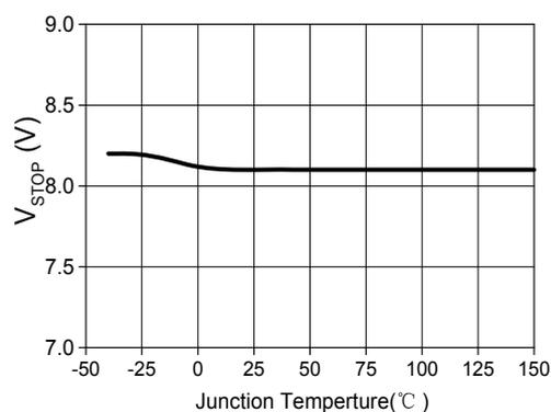
(d)  $V_{STOP}$  vs  $T_j$
