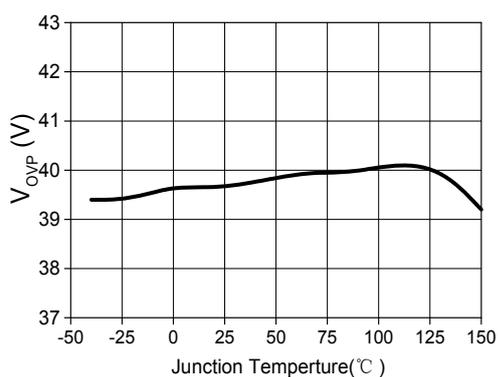
(e)  $V_{OVP}$  vs  $T_j$
