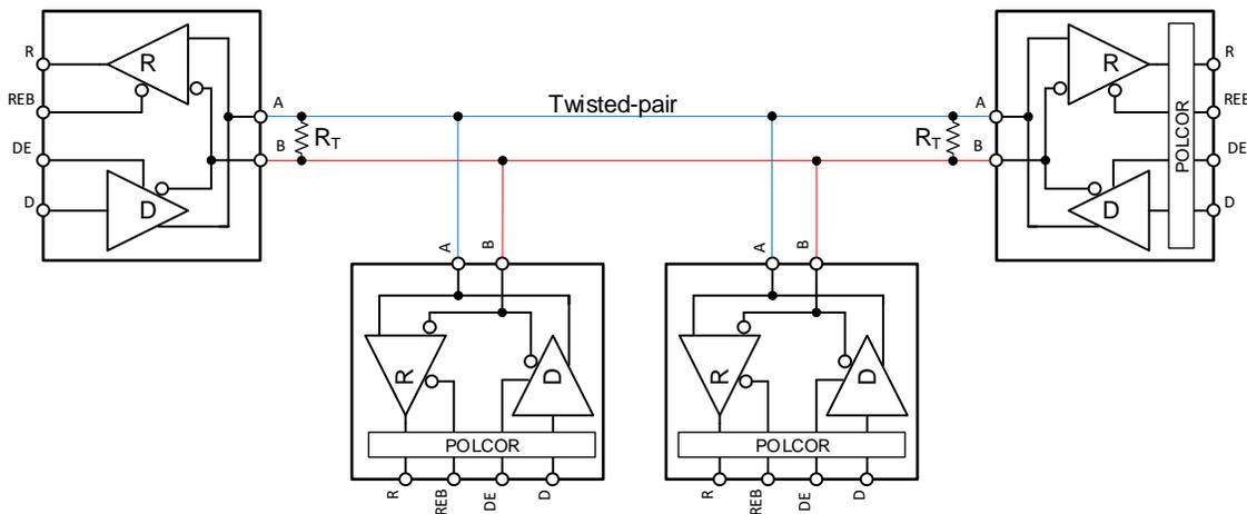
**Figure 10-1. Typical RS-485 Network With CS485xx Half-Duplex Transceivers**
