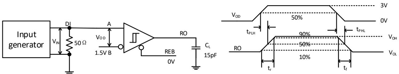
Figure 8-6. Receiver Output Rise and Fall Times and Propagation Delays
