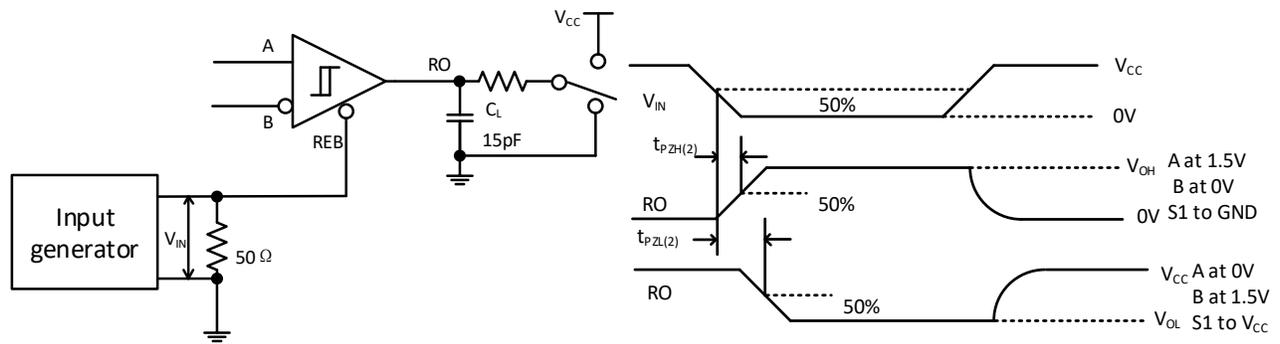
**Figure 8-8. Receiver Enable Times With Driver Disabled**
