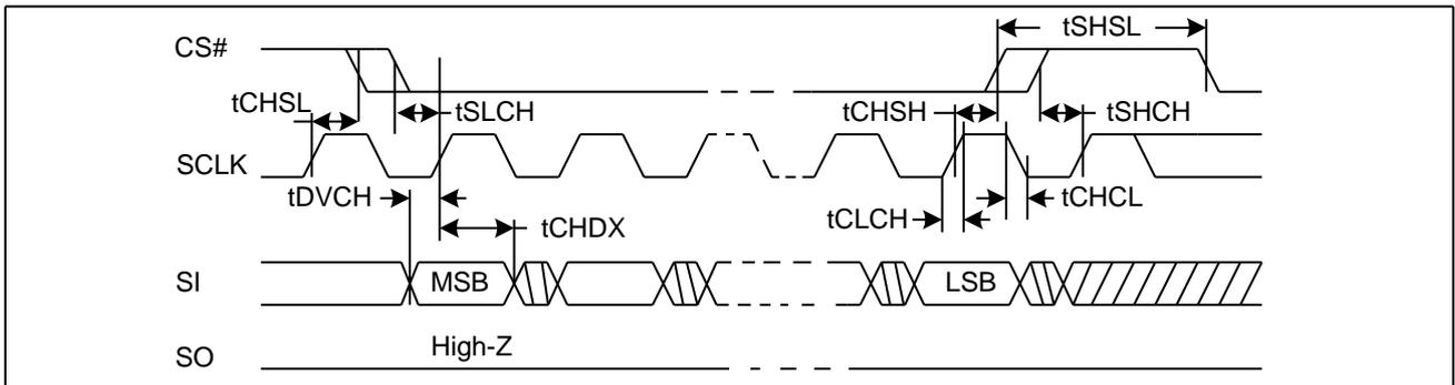
Figure20-2. Output Timing
