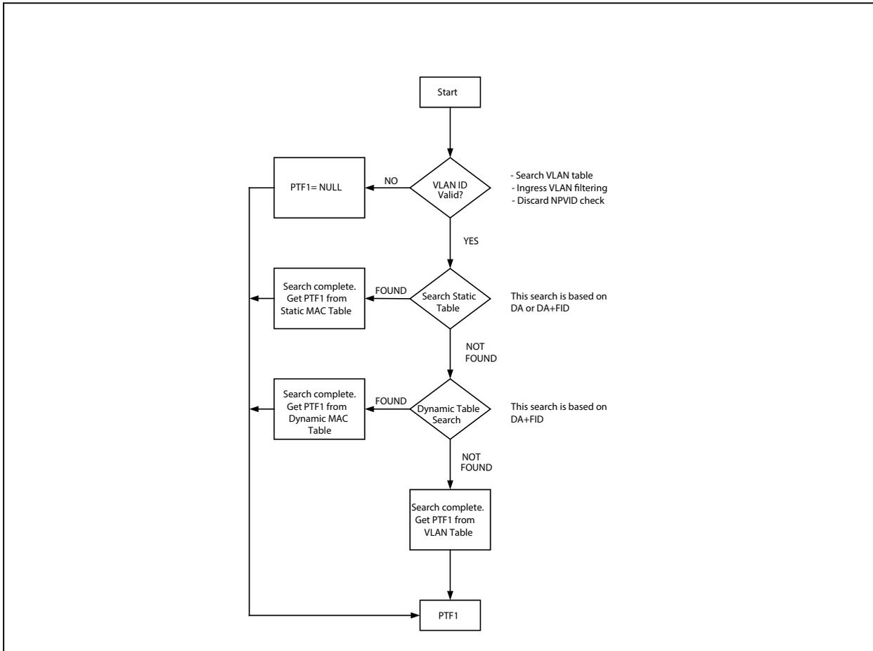
**FIGURE 3-5: DESTINATION ADDRESS RESOLUTION FLOW CHART, STAGE 2**
