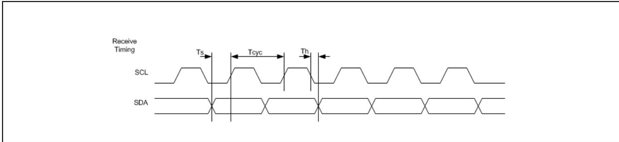
FIGURE 7-10: I<sup>2</sup>C START BIT TIMING
