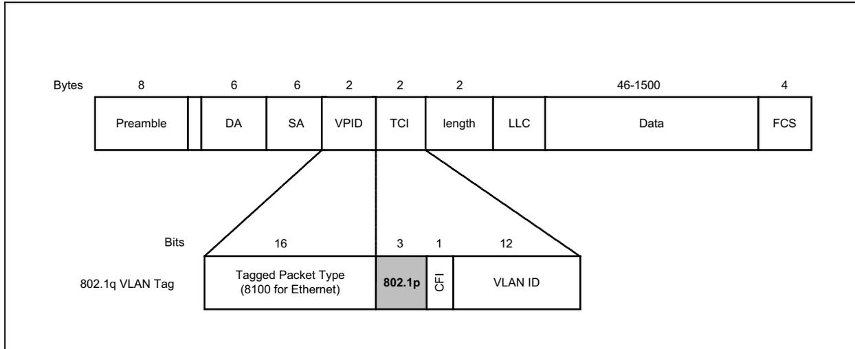
802.1p-based priority is enabled by bit [5] of registers 16, 32 and 48 for ports 1, 2 and 3, respectively.
