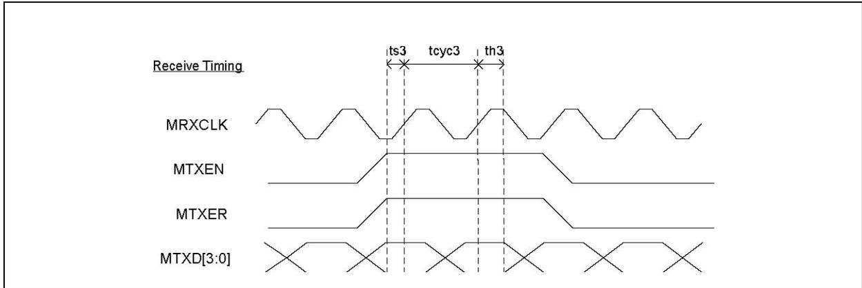
**FIGURE 7-4: MAC MODE MII TIMING - DATA TRANSMITTED TO MII**
