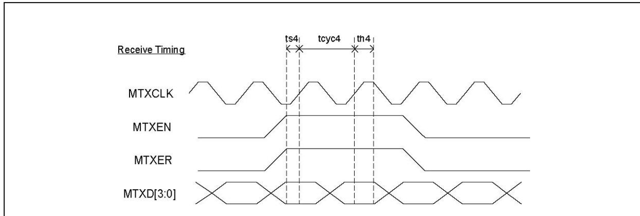
FIGURE 7-6: PHY MODE MII TIMING - DATA TRANSMITTED TO MII
