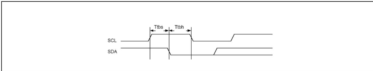
FIGURE 7-11: I<sup>2</sup>C STOP BIT TIMING
