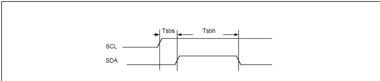
FIGURE 7-12: I<sup>2</sup>C OUTPUT TIMING
