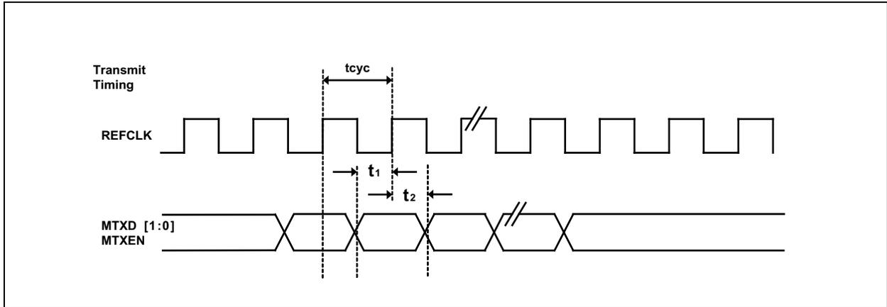
FIGURE 7-8: RMI TIMING - DATA TRANSMITTED TO RMI
