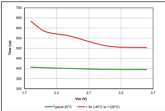
**FIGURE 38-44:** Wake From Sleep,  $LFINTOSC$ , PIC16LF18855/75 Only.
