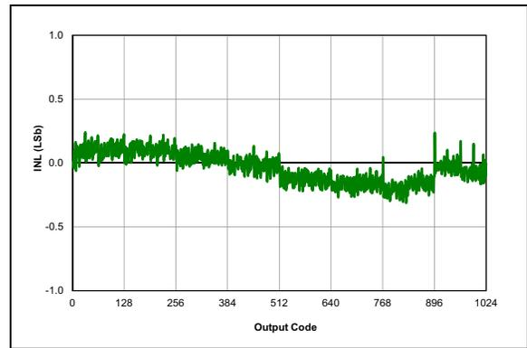
**FIGURE 38-47:** ADC, INL,  $V_{DD} = 3.0V$ ,  $T_{AD} = 1\ \mu\text{S}$ ,  $25^\circ\text{C}$ .
