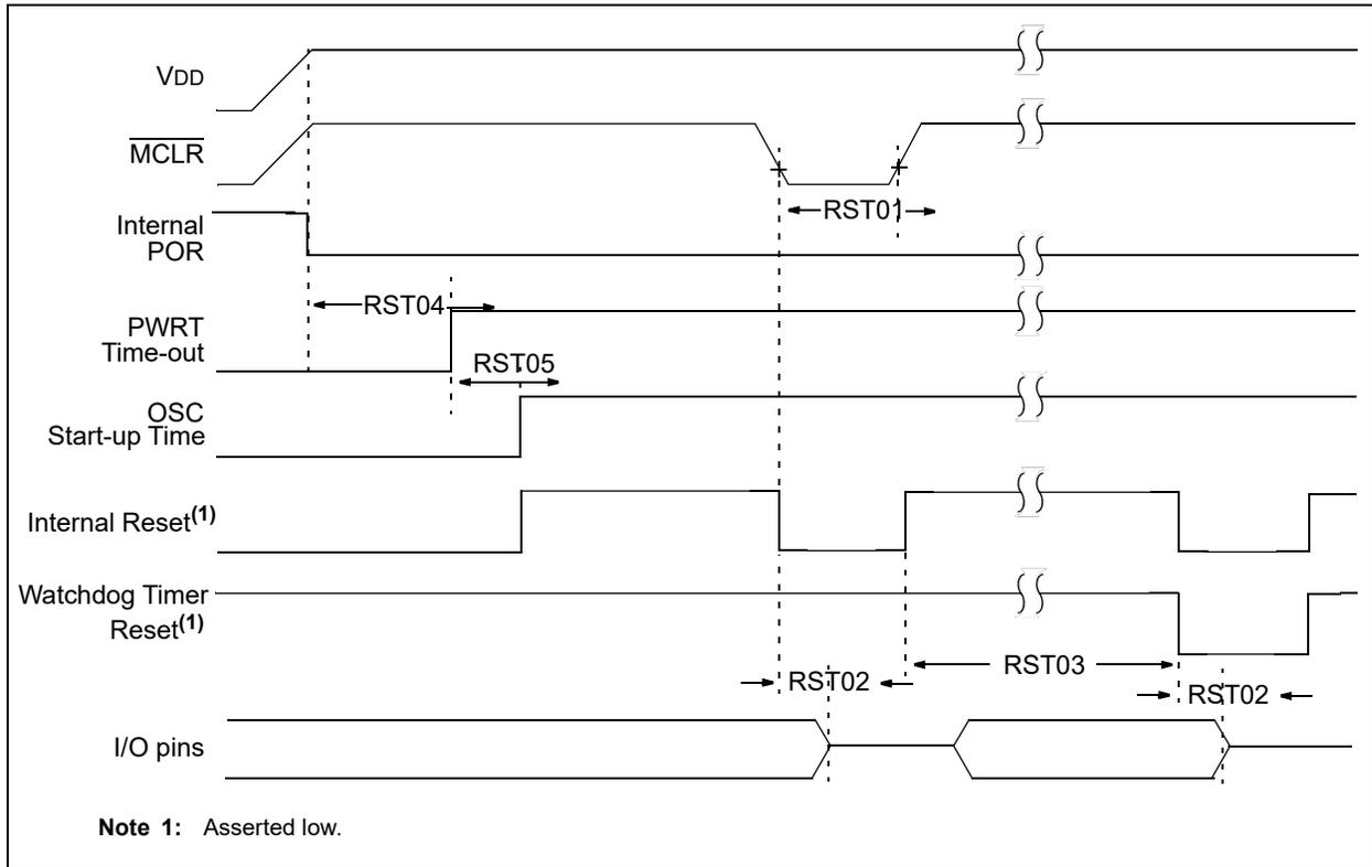
**FIGURE 37-9: BROWN-OUT RESET TIMING AND CHARACTERISTICS**
