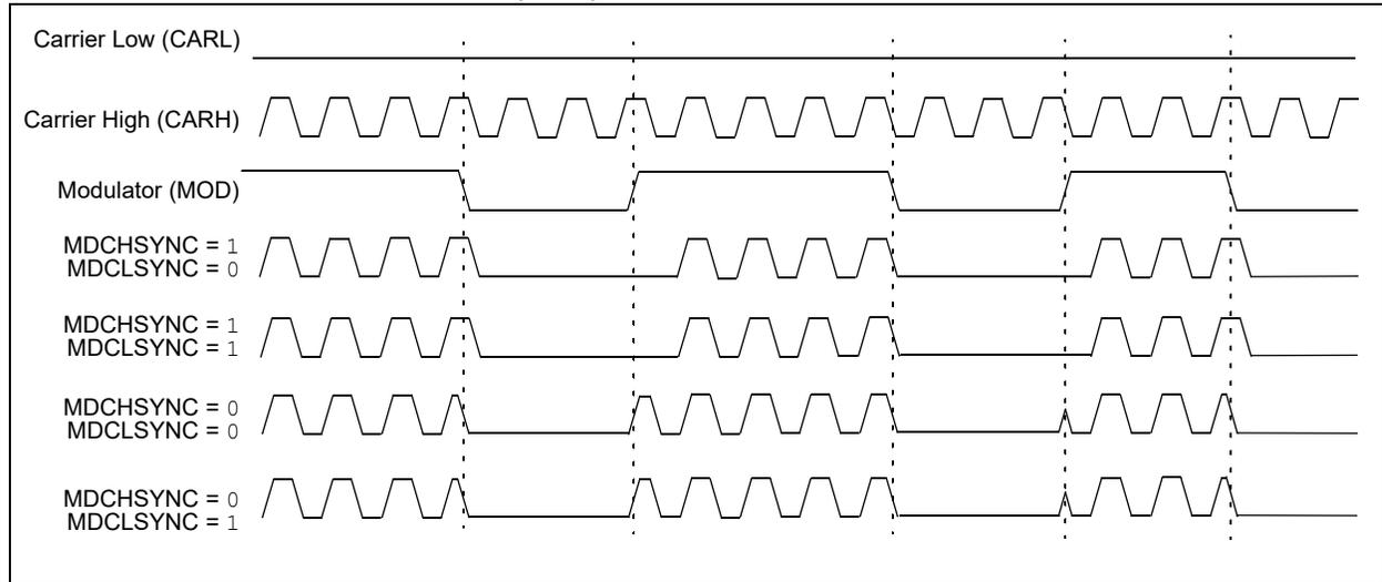
**FIGURE 26-3: NO SYNCHRONIZATION (MDSHSYNC = 0, MDCLSYNC = 0)**
