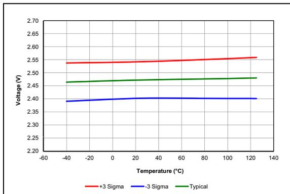
**FIGURE 38-27:** Brown-Out Reset Voltage, Trip Point (BORV = 1x).
