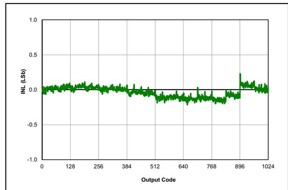
**FIGURE 38-48:** ADC, INL,  $V_{DD} = 3.0V$ ,  $T_{AD} = 4\ \mu\text{S}$ ,  $25^\circ\text{C}$ .
