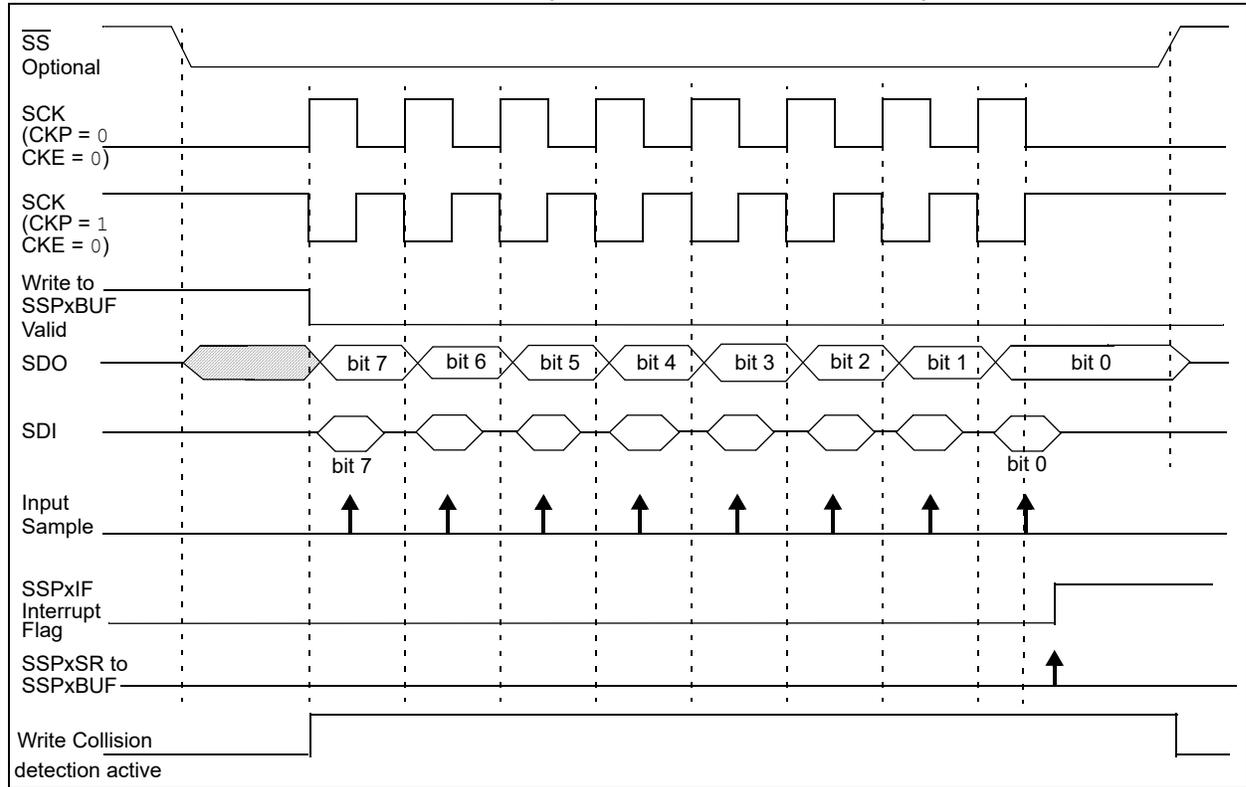
**FIGURE 31-10: SPI MODE WAVEFORM (CLIENT MODE WITH CKE = 1)**
