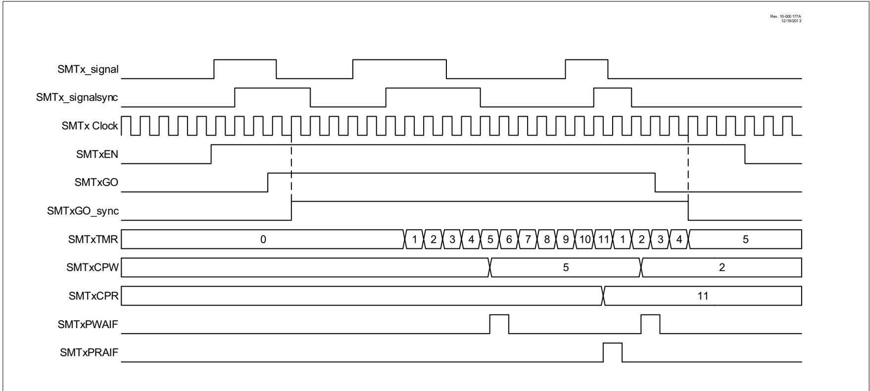
**FIGURE 32-7: PERIOD AND DUTY-CYCLE SINGLE ACQUISITION TIMING DIAGRAM**
