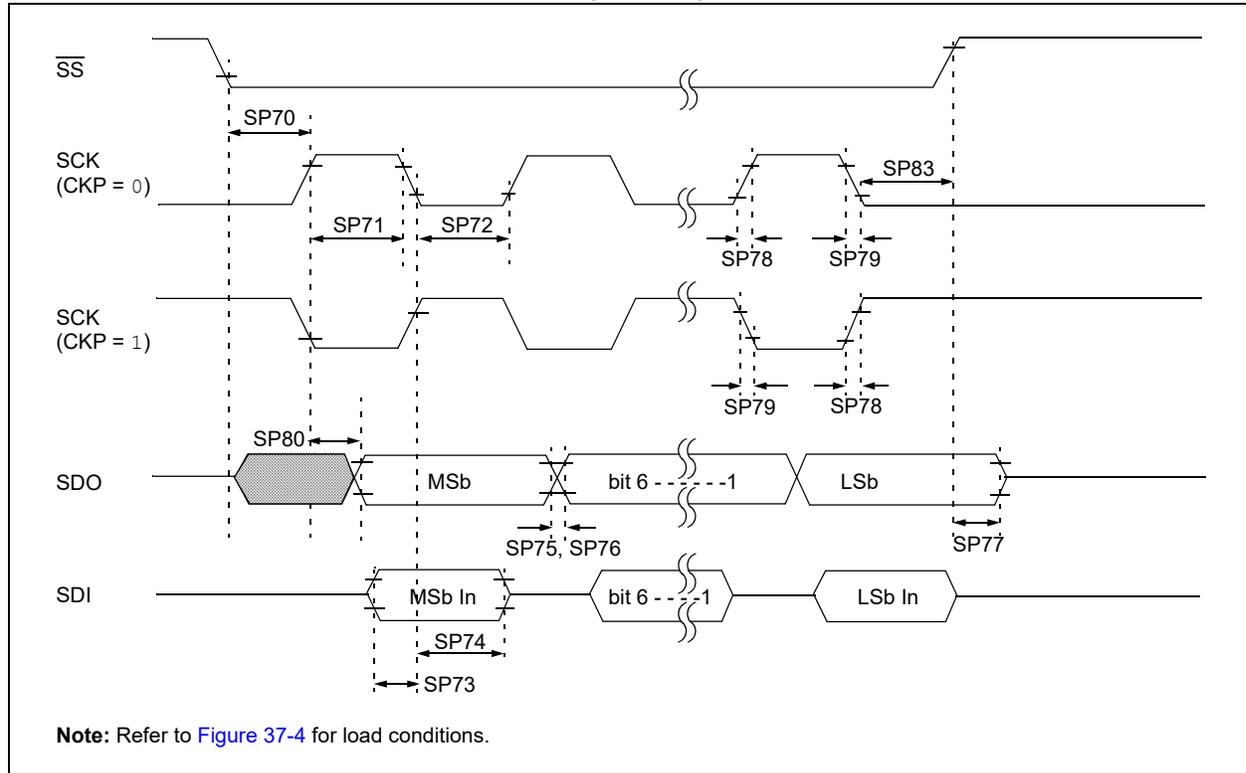
**FIGURE 37-20: SPI CLIENT MODE TIMING (CKE = 1)**
