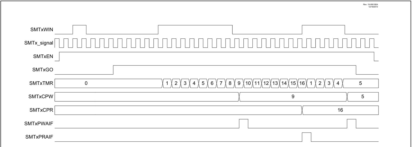
**FIGURE 32-22: WINDOWED COUNTER MODE SINGLE ACQUISITION TIMING DIAGRAM**
