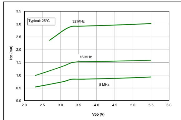
**FIGURE 38-5:**  $I_{DD}$ , ECH Oscillator, Typical, PIC16F18855/75 Only.
