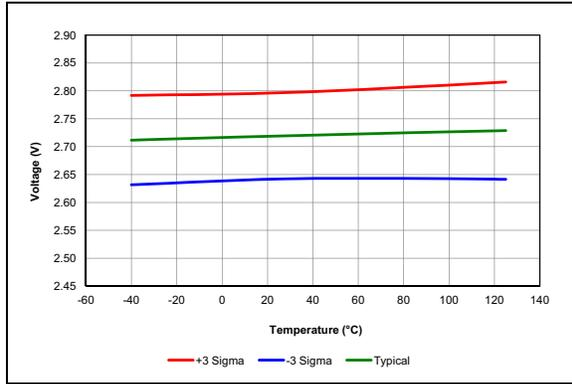
**FIGURE 38-25:** Brown-Out Reset Voltage, Trip Point (BORV = 01).
