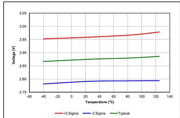
**FIGURE 38-23:** Brown-Out Reset Voltage, Trip Point (BORV = 00).
