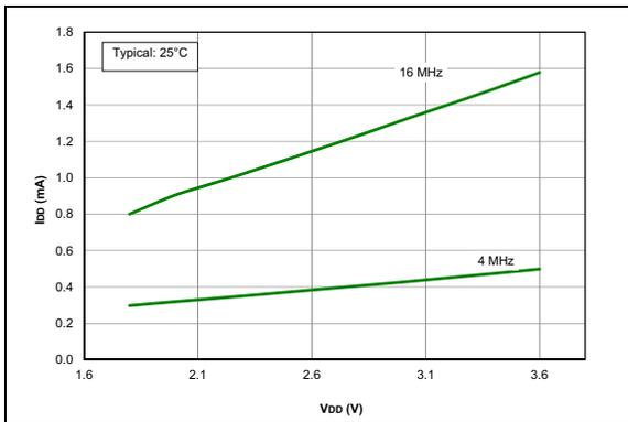
**FIGURE 38-8:**  $I_{DD}$  Typical, INT Oscillator, PIC16LF18855/75 Only.
