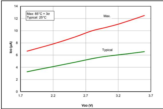
**FIGURE 38-7:**  $I_{DD}$ , LFINT,  $F_{osc} = 31\text{ kHz}$ , PIC16LF18855/75 Only.
