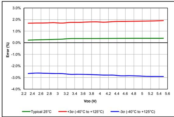
**FIGURE 38-91:** HFINTOSC Typical Frequency Error, PIC16F18855/75 Only.
