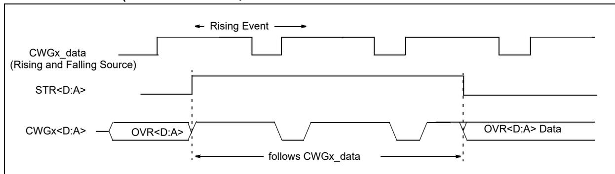
**FIGURE 20-11: EXAMPLE OF STEERING EVENT AT BEGINNING OF INSTRUCTION ( $MODE<2:0> = 001$ )**
