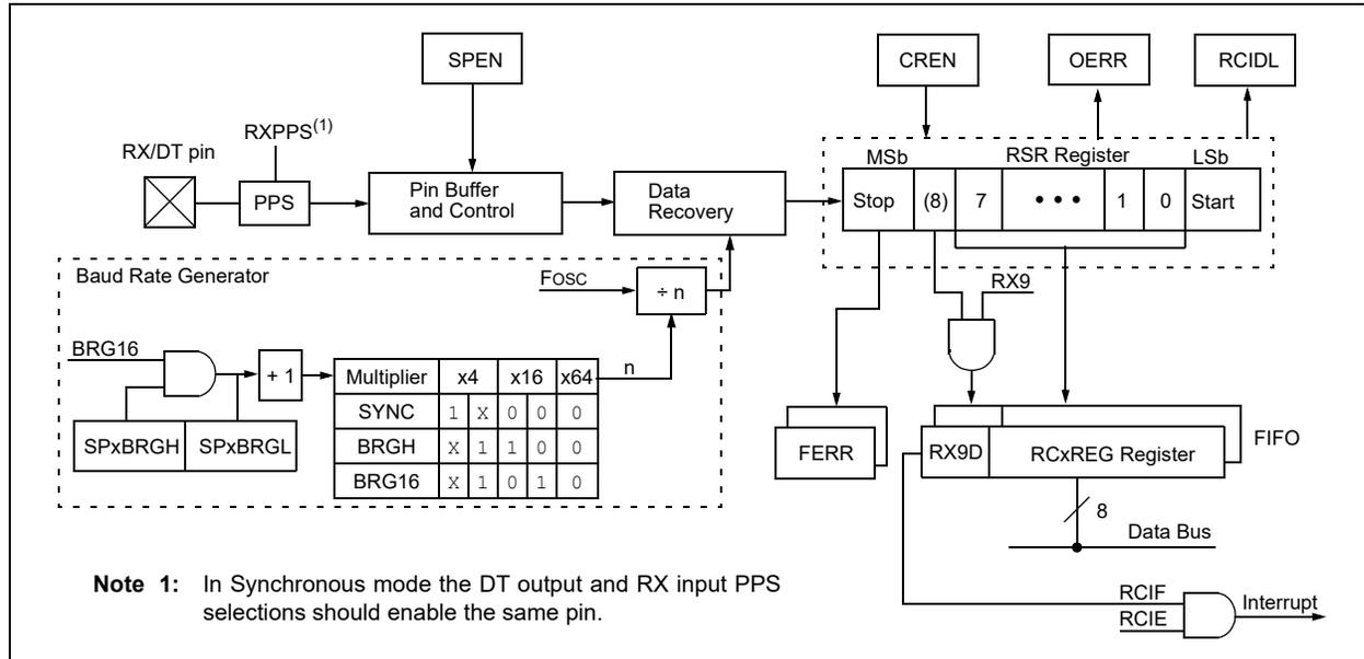
The operation of the EUSART module is controlled through three registers:
