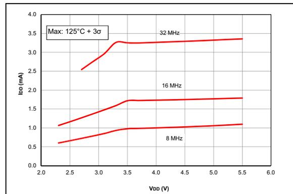
**FIGURE 38-6:**  $I_{DD}$ , ECH Oscillator, Maximum, PIC16F18855/75 Only.
