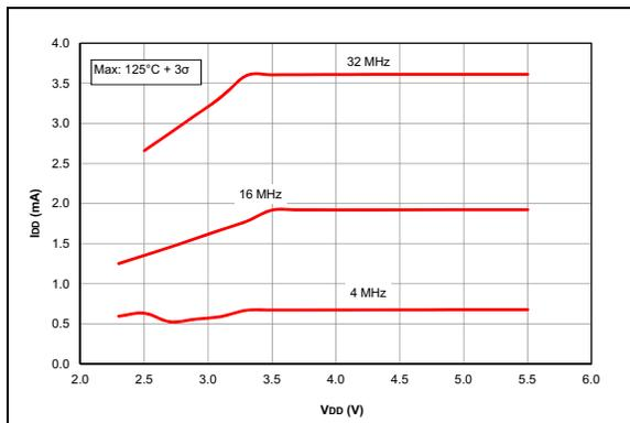
**FIGURE 38-3:**  $I_{DD}$  Maximum, INT Oscillator, PIC16F18855/75 Only.
