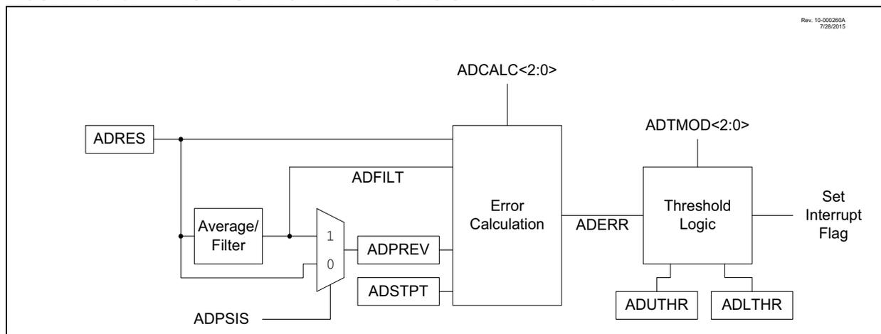
The operation of the ADC computational features is controlled by the ADMD <2:0> bits in the ADCON2 register.
