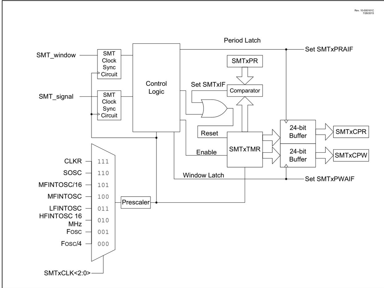
**FIGURE 32-2: SMT SIGNAL AND WINDOW BLOCK DIAGRAM**
