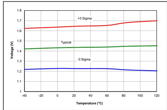
**FIGURE 38-36:** POR Rearm Voltage, VREGPM1 = 0, PIC16F18855/75 Only.
