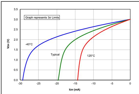
**FIGURE 38-15:**  $V_{OH}$  vs.  $I_{OH}$  Over Temperature,  $V_{DD} = 3.0V$ .
