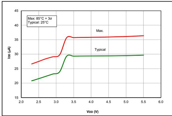
**FIGURE 38-1:**  $I_{DD}$ , LFINT,  $F_{osc} = 31\text{ kHz}$ , PIC16F18855/75 Only.
