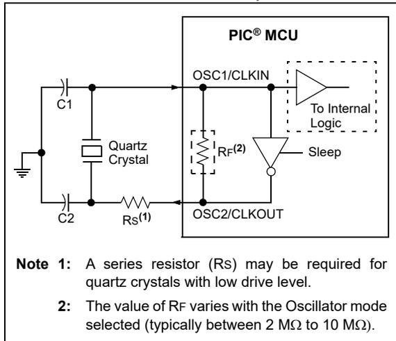
**Note 1:** Quartz crystal characteristics vary according to type, package and manufacturer. The user should consult the manufacturer data sheets for specifications and recommended application.
