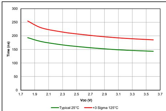
**FIGURE 38-80:** Comparator Response Time, Falling Edge, PIC16LF18855/75 Only.
