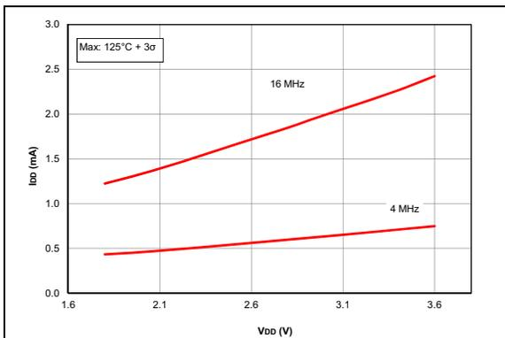
**FIGURE 38-9:**  $I_{DD}$  Maximum, INT Oscillator, PIC16LF18855/75 Only.
