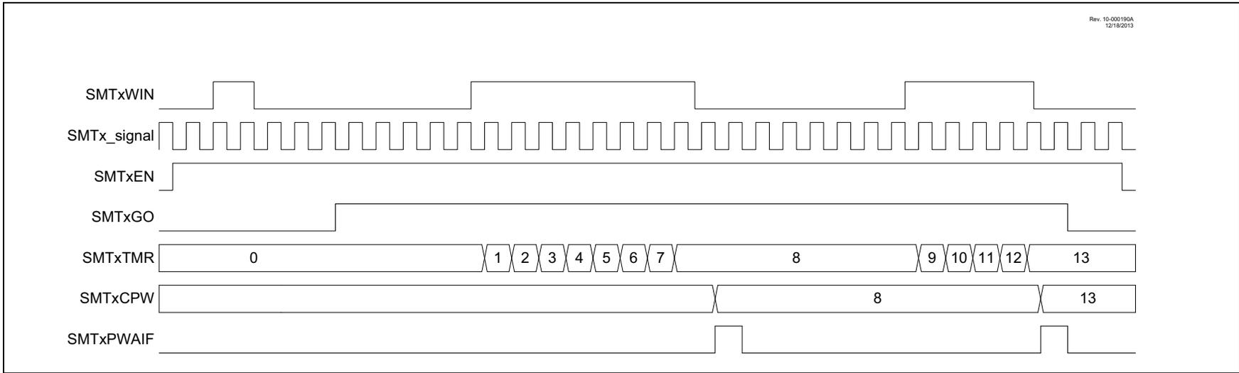
**FIGURE 32-20: GATED COUNTER MODE SINGLE ACQUISITION TIMING DIAGRAM**
