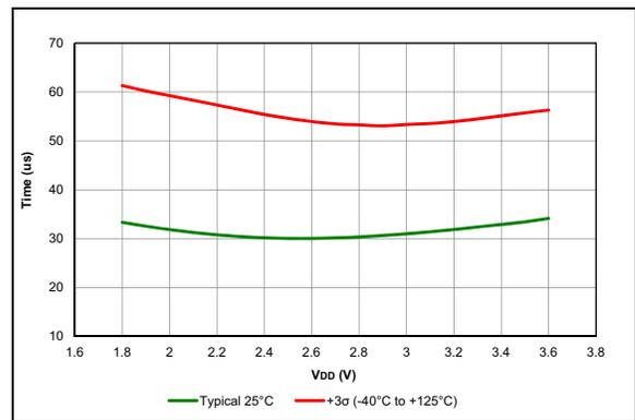
**FIGURE 38-77:** Band Gap Ready Time, PIC16LF18855/75 Only.
