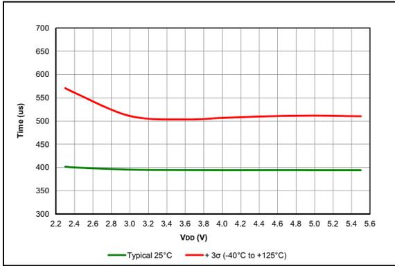
**FIGURE 38-43:** Wake From Sleep,  $V_{REGPM} = 1$ ,  $LFINTOSC$ , PIC16F18855/75 Only.
