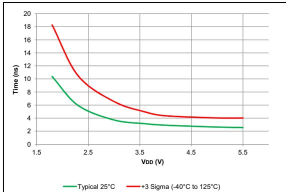
**FIGURE 38-99:** Fall Time, Slew Rate Control Disabled.
