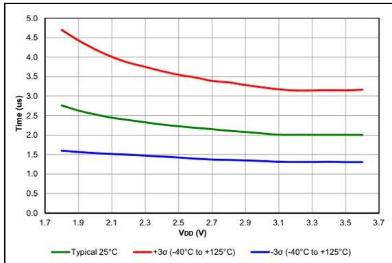
**FIGURE 38-75:** ADC RC Oscillator Period, PIC16LF18855/75 Only.
