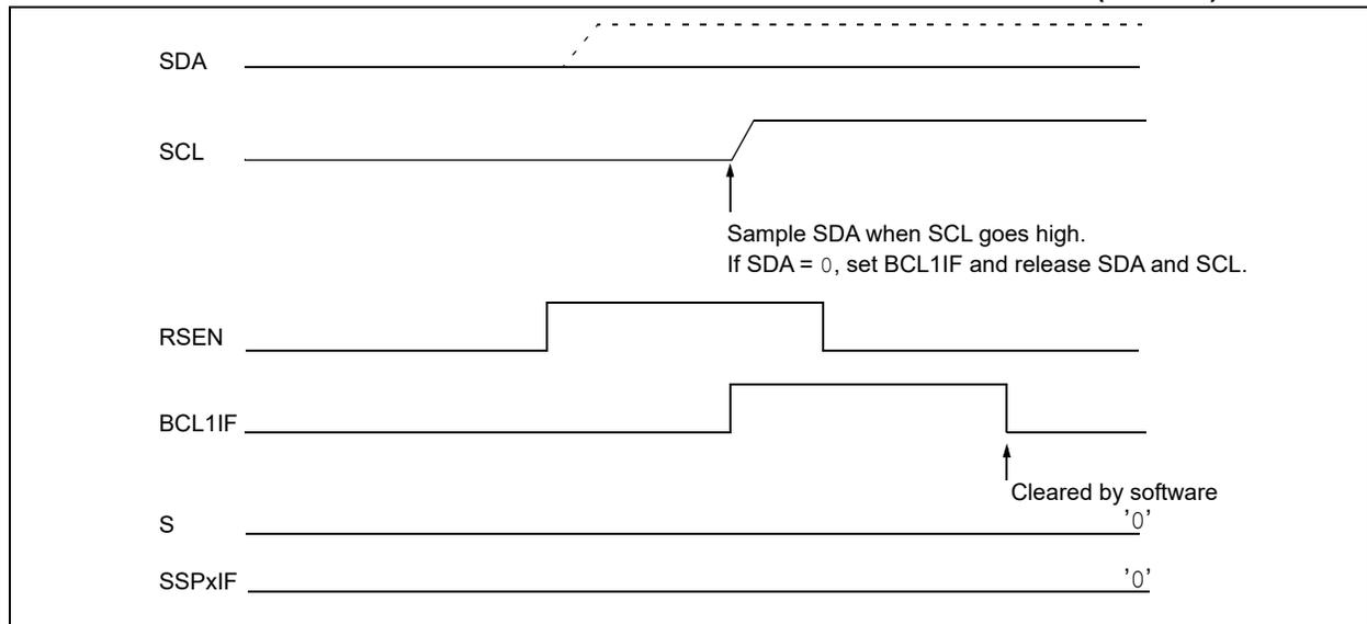
**FIGURE 31-37: BUS COLLISION DURING REPEATED START CONDITION (CASE 2)**
