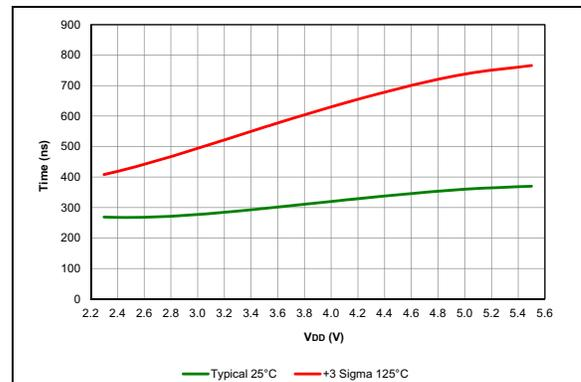
**FIGURE 38-83:** Comparator Response Time, Rising Edge, PIC16F18855/75 Only.
