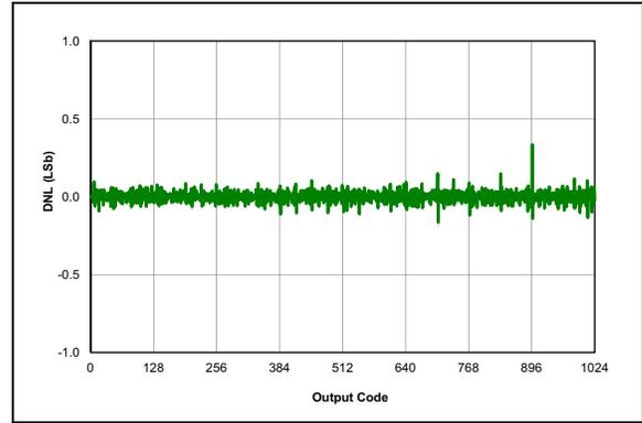
**FIGURE 38-46:** ADC, DNL,  $V_{DD} = 3.0V$ ,  $T_{AD} = 4\ \mu\text{S}$ ,  $25^\circ\text{C}$ .
