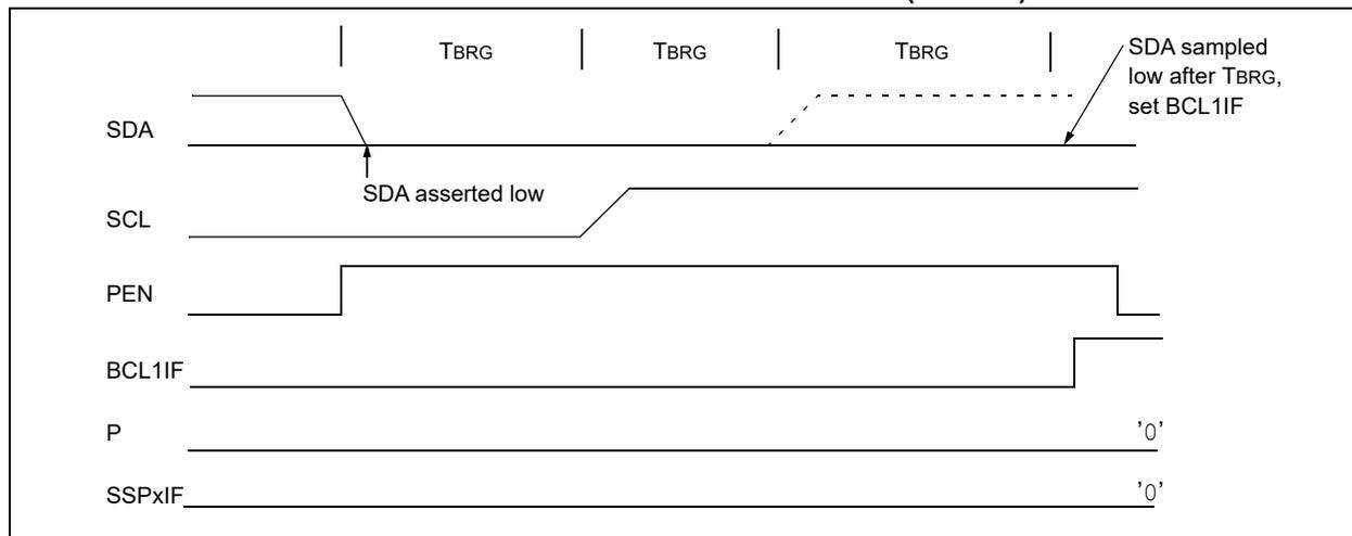
**FIGURE 31-39: BUS COLLISION DURING A STOP CONDITION (CASE 2)**
