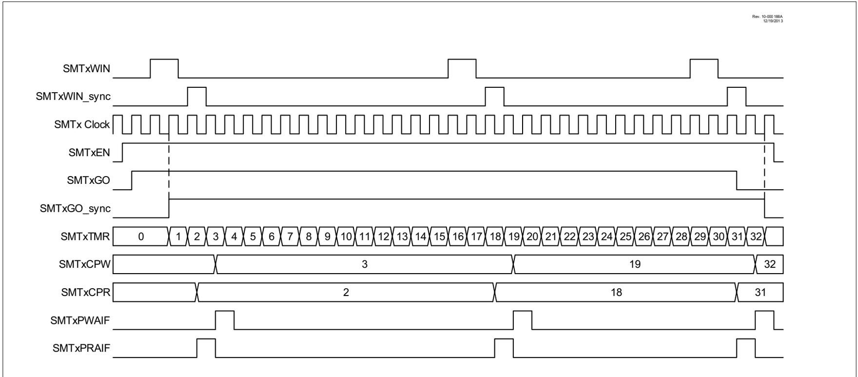
**FIGURE 32-17: CAPTURE MODE SINGLE ACQUISITION TIMING DIAGRAM**
