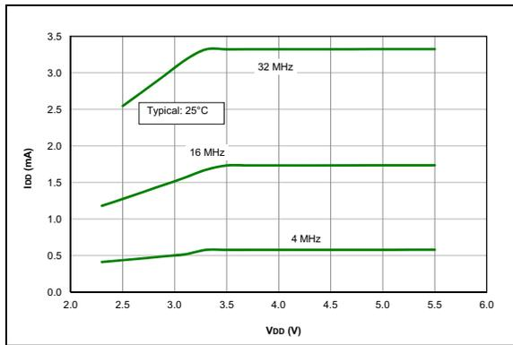
**FIGURE 38-2:**  $I_{DD}$  Typical, INT Oscillator, PIC16F18855/75 Only.
