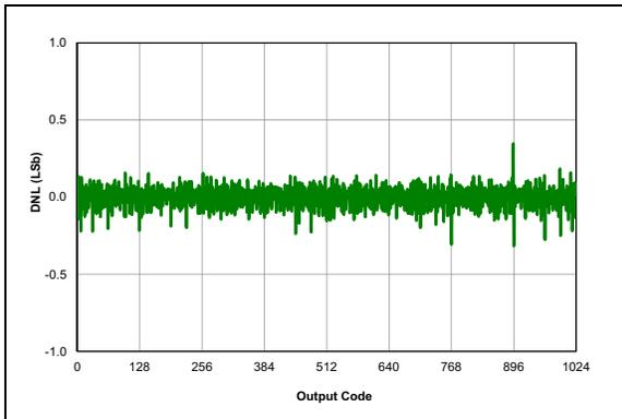
**FIGURE 38-45:** ADC, DNL,  $V_{DD} = 3.0V$ ,  $T_{AD} = 1\ \mu\text{S}$ ,  $25^\circ\text{C}$ .
