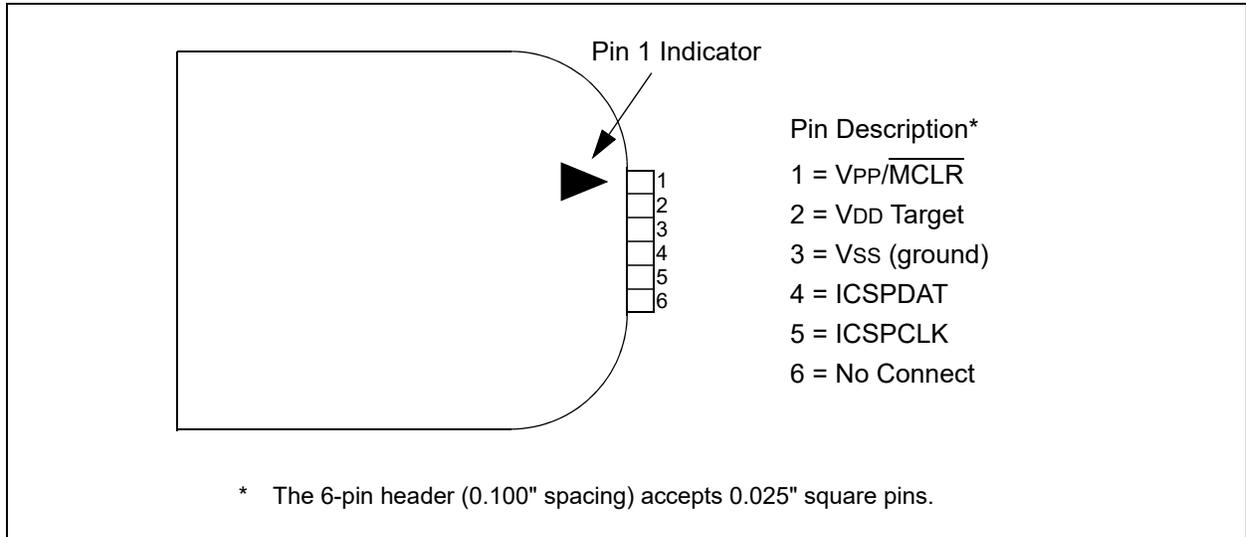
**FIGURE 35-3: TYPICAL CONNECTION FOR ICSP™ PROGRAMMING**
