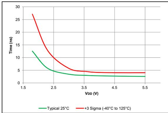
**FIGURE 38-98:** Rise Time, Slew Rate Control Disabled.
