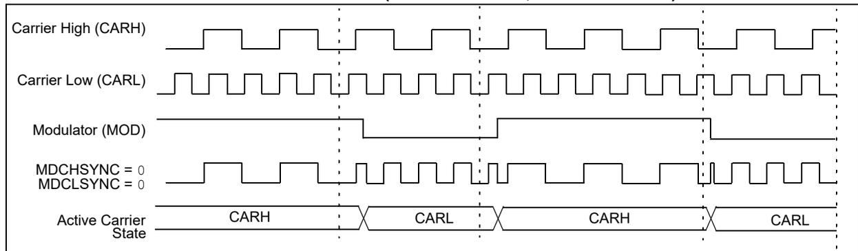
**FIGURE 26-4: CARRIER HIGH SYNCHRONIZATION (MDSHSYNC = 1, MDCLSYNC = 0)**
