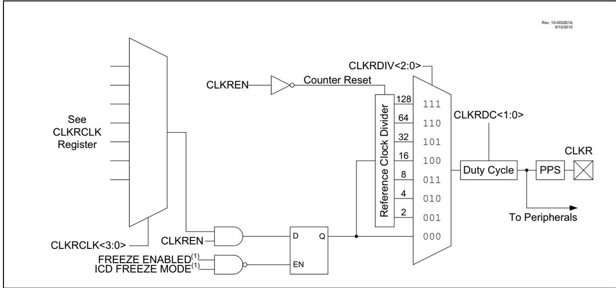
**FIGURE 34-2: CLOCK REFERENCE TIMING**
