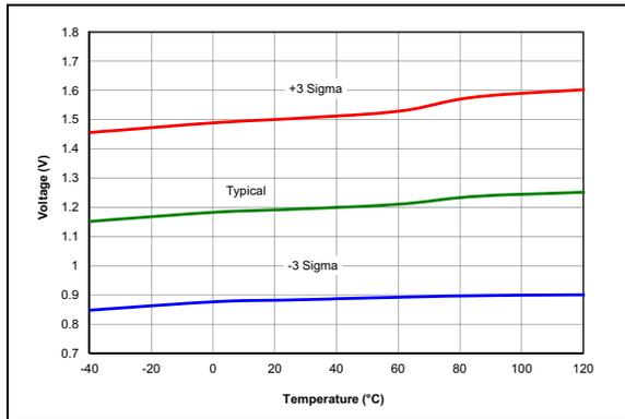
**FIGURE 38-37:** POR Rearm Voltage,  $V_{REGPM1} = 1$ , PIC16F18855/75 Only.
