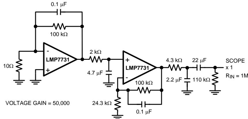
**Figure 45. 0.1 Hz to 10 Hz Noise Test Circuit**
