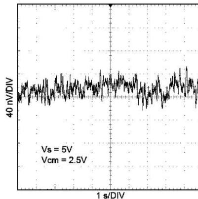
**Figure 46. 0.1 Hz to 10 Hz Input Voltage Noise**
