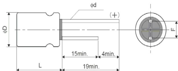
**Lead Spacing, diameter and size code**
