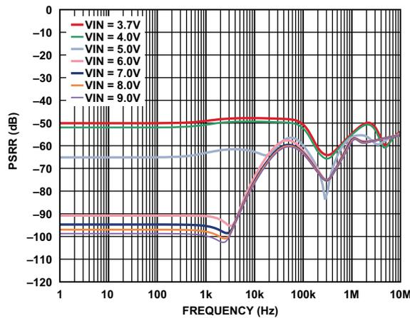
Figure 6. VOUT1 PSRR,  $I_{\text{OUT1}} = 40\ \text{mA}$
