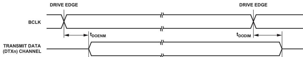
Figure 13. I<sup>2</sup>S Slave (A<sup>2</sup>B Main Node) Enable and Three-State Timing
