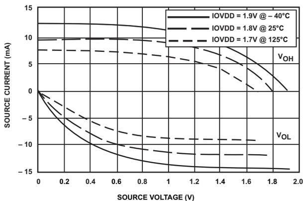
Figure 25. Digital I/O Drivers (DS1, 1.8 V IOVDD)
