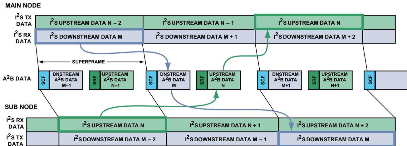
Figure 4. A<sup>2</sup>B Bus Synchronous Data Exchange
