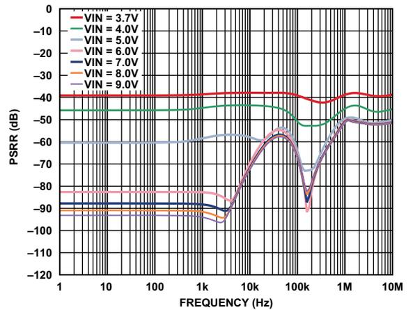
Figure 8. VOUT2 PSRR,  $I_{\text{OUT2}} = 50\ \text{mA}$
