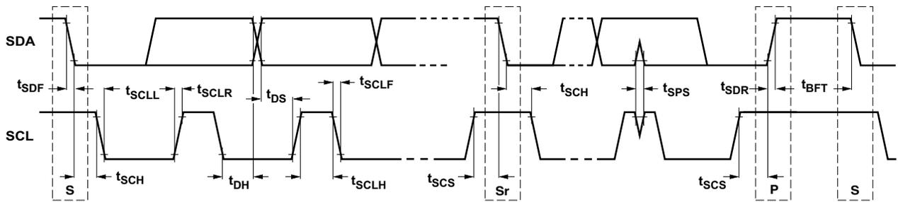
Figure 10. I<sup>2</sup>C Port Timing
