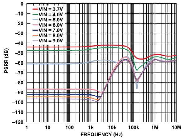
Figure 7. VOUT2 PSRR,  $I_{\text{OUT2}} = 10\ \text{mA}$
