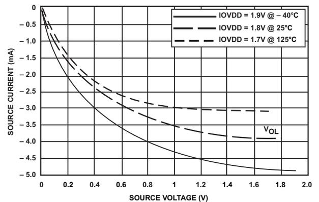
Figure 23. I<sup>2</sup>C Drivers (1.8 V IOVDD)
