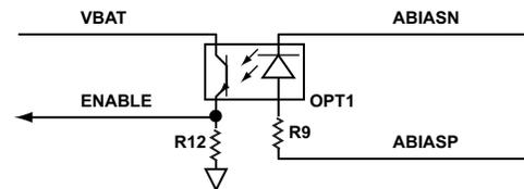
*Figure 38. Optional Power Supply Enable Circuit with Optocoupler*
