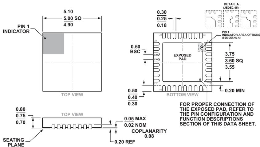
Figure 41. 32-Lead Lead Frame Chip Scale Package [LFCSP]
