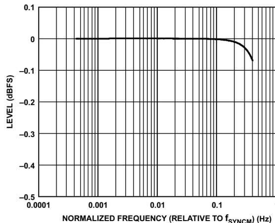
Figure 16. PDM Frequency Response,  $f_{\text{SYNC}} = 48 \text{ kHz}$
