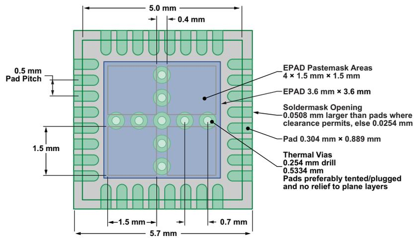
Figure 39. Transceiver Footprint
