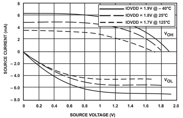
Figure 21. Digital I/O Drivers (DS0, 1.8 V IOVDD)
