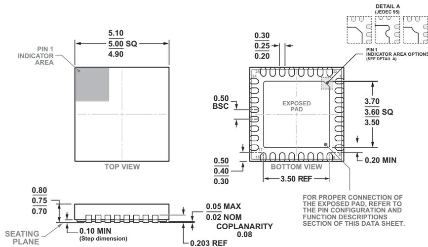
Figure 40. 32-Lead Lead Frame Chip Scale Package [LFCSP\_SS]
