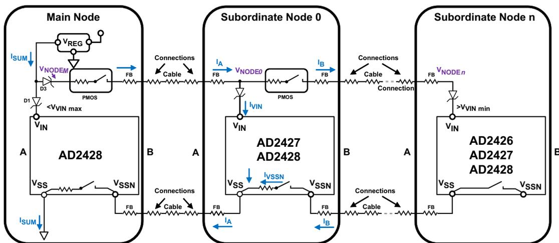
Figure 37. A<sup>2</sup>B Power Model for Bus Powered System
