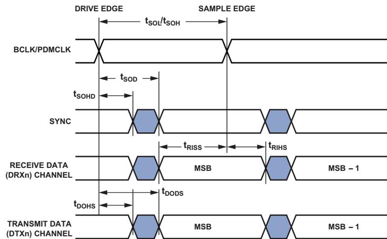
Figure 12. I<sup>2</sup>S Master (A<sup>2</sup>B Subordinate Node) Timing
