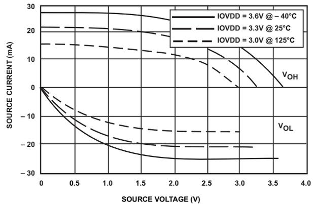
Figure 22. Digital I/O Drivers (DS0, 3.3 V IOVDD)
