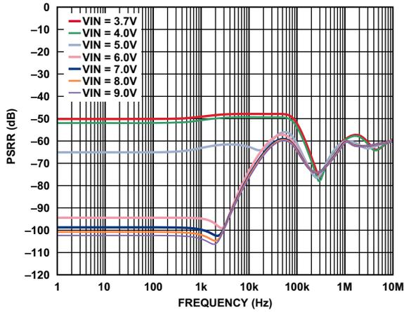
Figure 5. VOUT1 PSRR,  $I_{\text{OUT1}} = 10\ \text{mA}$
