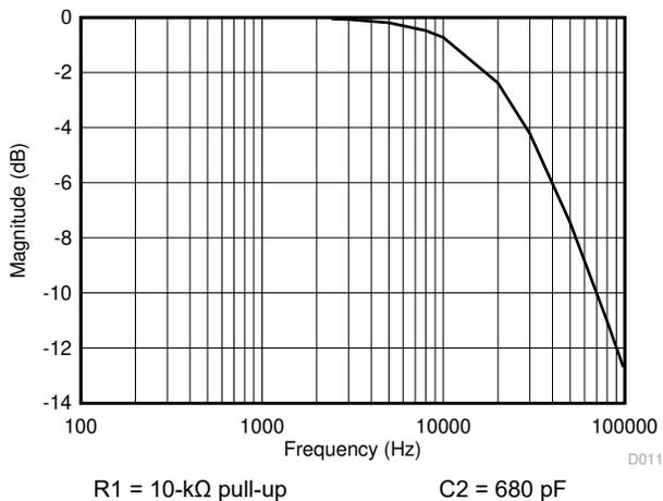
**Figure 8-4. Low-Pass Filtering**
