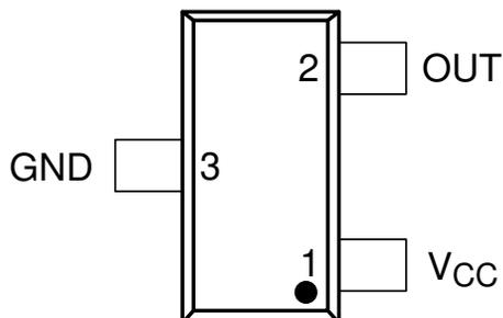
Figure 5-1. DBZ Package 3-Pin SOT-23 Top View
