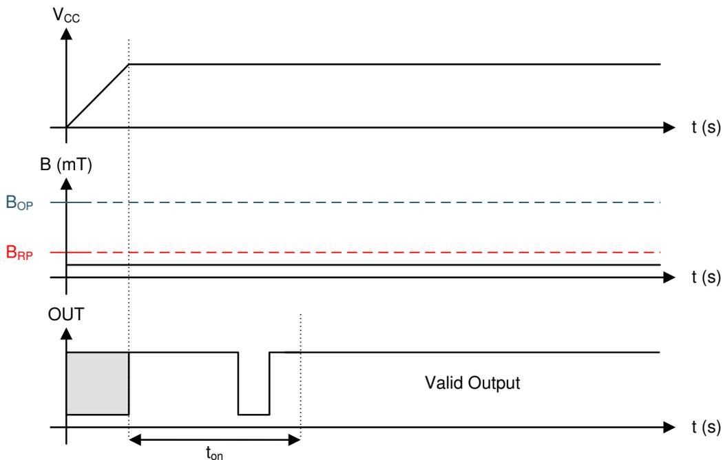
Figure 7-4. Case 2: Power On When  $B < B_{RP}$
