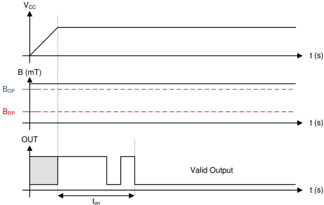
Figure 7-3. Case 1: Power On When  $B > B_{OP}$
