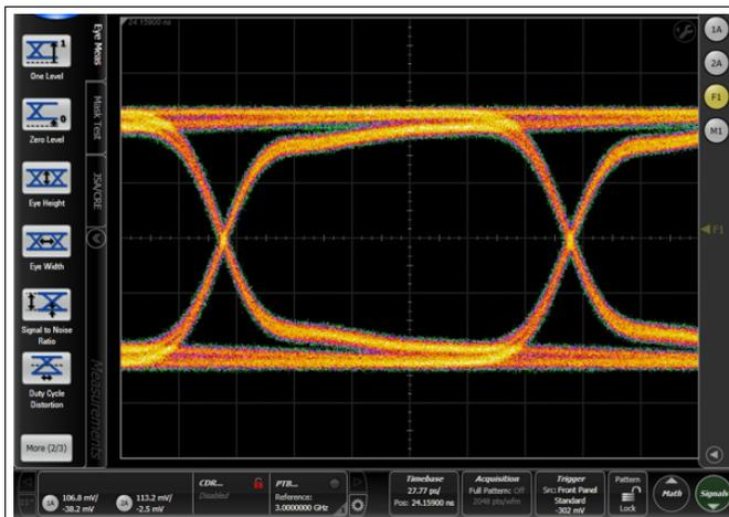
Figure 13. HDMI 2.0 6 Gbps Eye Diagram (Bare Board)
