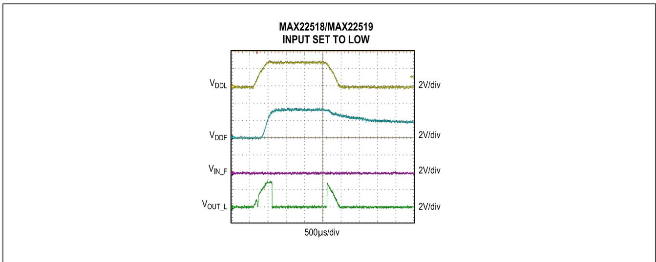
Figure 6. Undervoltage Lockout Behavior (MAX22518/MAX22519, Input Low)
