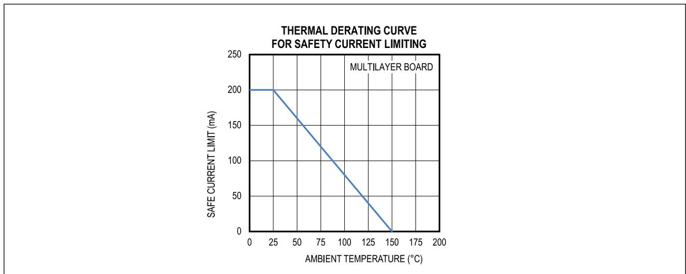
Figure 8. Thermal Derating Curve for Safety Current Limiting
