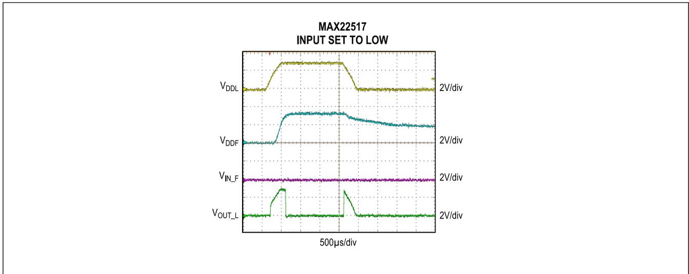
Figure 5. Undervoltage Lockout Behavior (MAX22517, Input Low)
