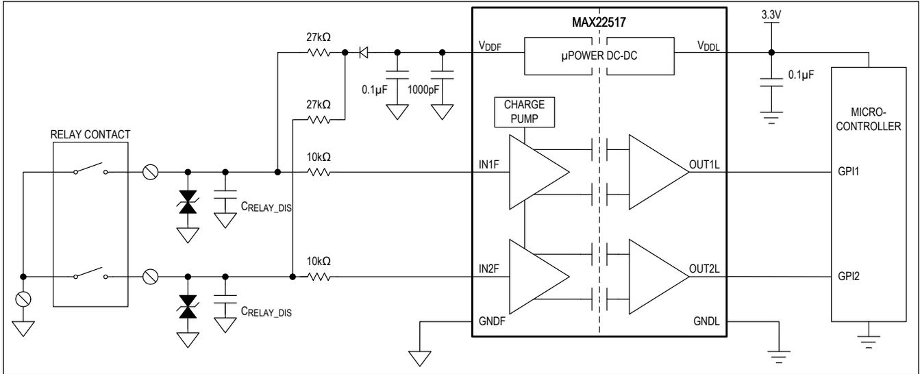
Single-Channel Relay Contact Monitoring With Self-Diagnostics
