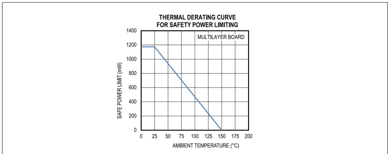
Figure 7. Thermal Derating Curve for Safety Power Limiting
