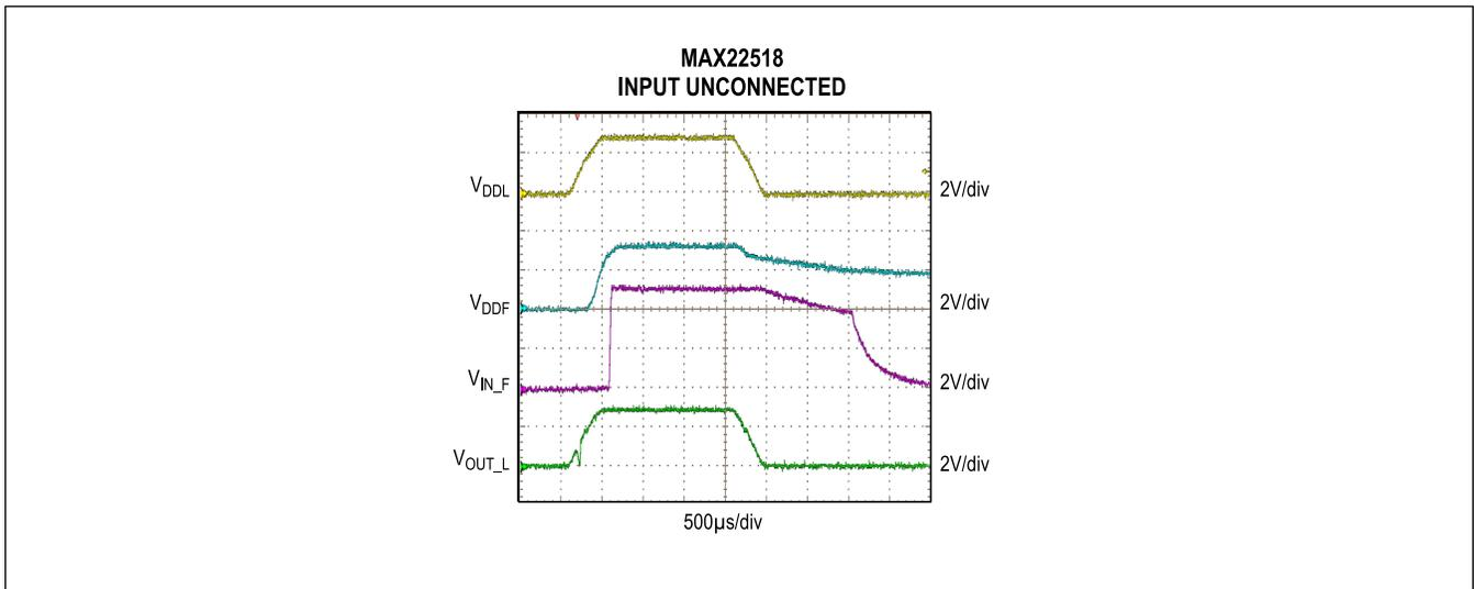
Figure 4. Undervoltage Lockout Behavior (MAX22518, Input Unconnected)
