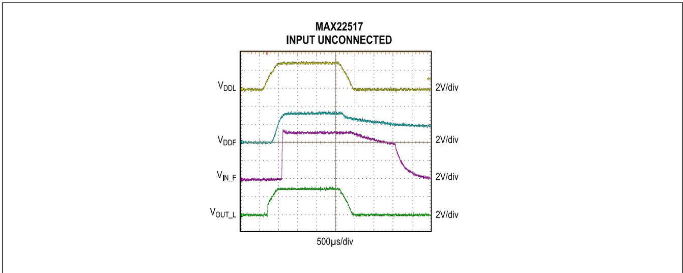
Figure 3. Undervoltage Lockout Behavior (MAX22517, Input Unconnected)
