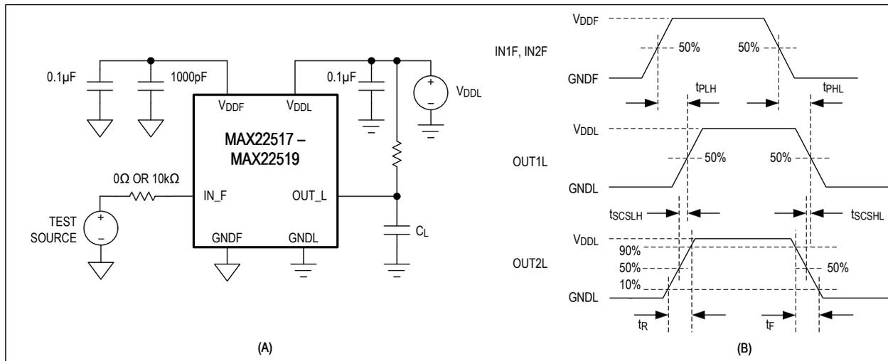
Figure 1. Test Circuit (A) and Timing Diagram (B)
