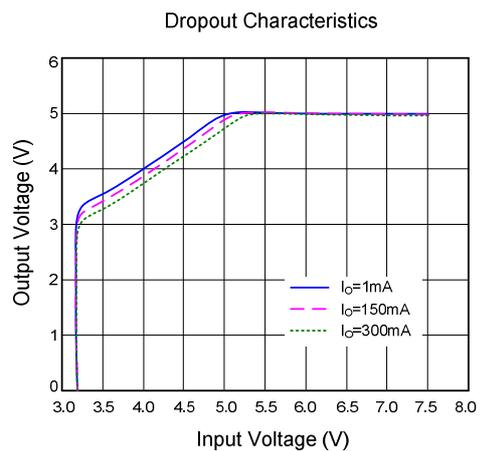
Figure 2. Dropout Characteristics
