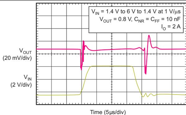
$V_{IN} = 1.4\text{ V to } 6\text{ V to } 1.4\text{ V at } 1\text{ V}/\mu\text{s}$ ,
