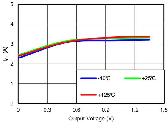
$V_{IN} = 1.8\text{ V}$ , ANY-OUT,  $V_{BIAS} = \text{Open}$ ,  $V_{OUT(TARGET)} = 1.5\text{ V}$
