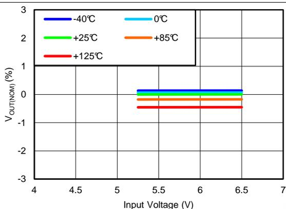
$V_{OUT(TARGET)} = 5\text{ V}$ ,  $I_{OUT} = 5\text{ mA}$ ,  $V_{BIAS} = \text{Open}$
