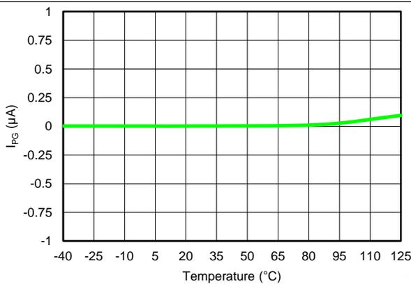
$V_{OUT(TARGET)} = 0.8\text{ V}$ ,  $V_{IN} = V_{PG} = 6.5\text{ V}$ ,  $V_{BIAS} = \text{Open}$
