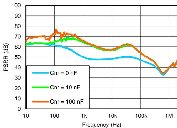
$V_{OUT(TARGET)} = 3.3\text{ V}$ , ANY-OUT,  $V_{IN} = V_{EN} = 3.8\text{ V}$ ,  $V_{BIAS} = \text{Open}$ ,  $I_{OUT} = 1.5\text{ A}$ ,  $C_{OUT} = 22\ \mu\text{F}$ ,  $C_{FF} = 10\text{ nF}$
