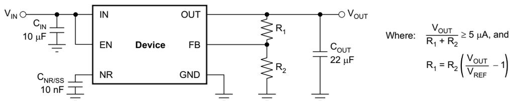
**Figure 50. Adjustable Operation for Maximum AC Performance**
