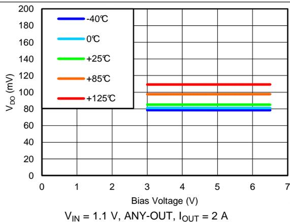
Figure 17. Minimum  $V_{IN}$  Dropout Voltage vs Bias Voltage
