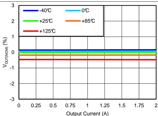
$V_{OUT(TARGET)} = 5\text{ V}$ ,  $V_{IN} = 5.3\text{ V}$ ,  $V_{BIAS} = \text{Open}$
