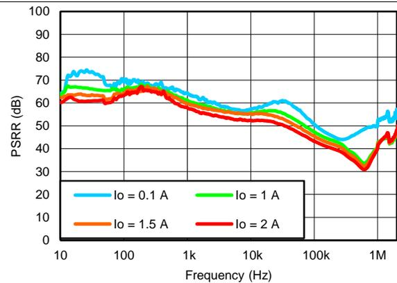
$V_{OUT(TARGET)} = 3.3\text{ V}$ , ANY-OUT,  $V_{IN} = V_{EN} = 3.8\text{ V}$ ,  $V_{BIAS} = \text{Open}$ ,  $C_{OUT} = 22\ \mu\text{F}$ ,  $C_{NR/SS} = C_{FF} = 10\text{ nF}$
