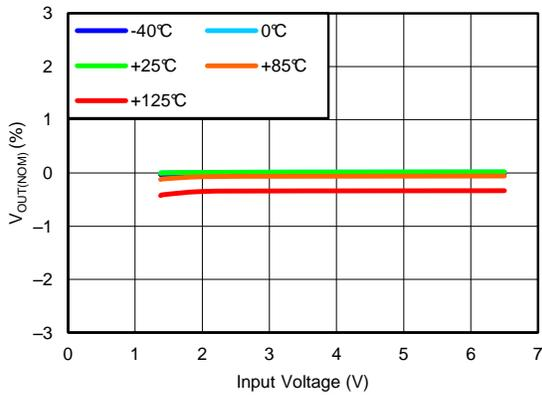
$V_{OUT(TARGET)} = 0.8\text{ V}$ ,  $I_{OUT} = 5\text{ mA}$ ,  $V_{BIAS} = \text{Open}$
