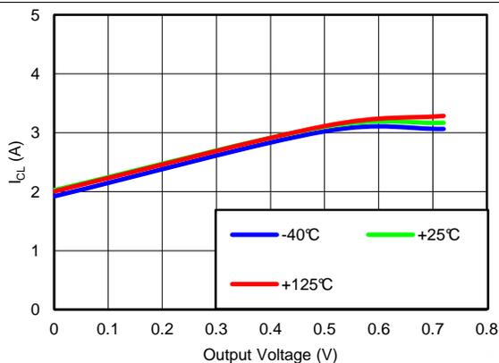
$V_{OUT(TARGET)} = 0.8\text{ V}$ ,  $V_{IN} = 1.1\text{ V}$ ,  $V_{BIAS} = 3\text{ V}$
