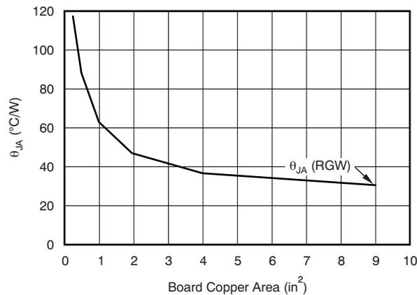
NOTE: The θ<sub>JA</sub> value at a board size of 9-in<sup>2</sup> (that is, 3-in × 3-in) is a JEDEC standard.
