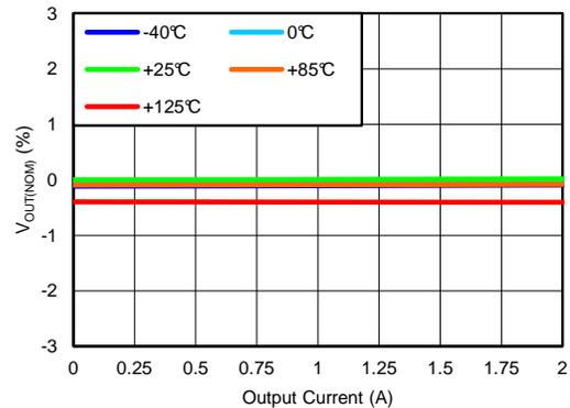
$V_{OUT(TARGET)} = 3.95\text{ V}$ ,  $V_{IN} = 4.25\text{ V}$ ,  $V_{BIAS} = \text{Open}$
