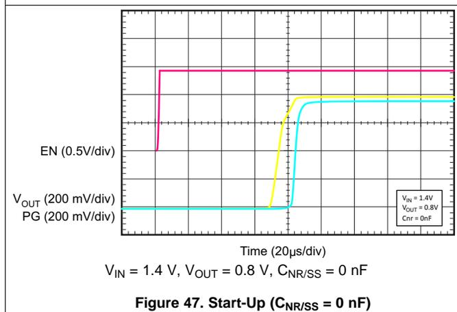
Figure 47. Start-Up ( $C_{NR/SS} = 0\text{ nF}$ )
