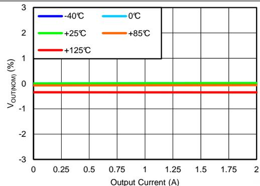
$V_{OUT(TARGET)} = 0.8\text{ V}$ ,  $V_{IN} = 1.1\text{ V}$ ,  $V_{BIAS} = 3\text{ V}$
