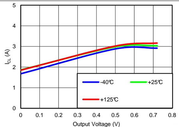
$V_{OUT(TARGET)} = 0.8\text{ V}$ ,  $V_{IN} = 1.1\text{ V}$ ,  $V_{BIAS} = 6.5\text{ V}$
