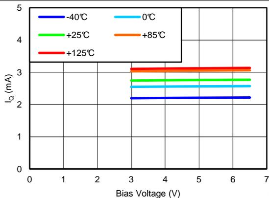
$V_{OUT(TARGET)} = 0.8\text{ V}$ ,  $I_{OUT} = 5\text{ mA}$ ,  $V_{IN} = 1.1\text{ V}$
