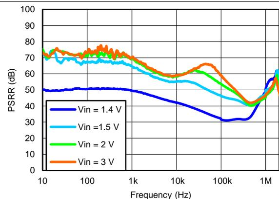
$V_{OUT(TARGET)} = 1.2\text{ V}$ , ANY-OUT,  $V_{BIAS} = \text{Open}$ ,  $I_{OUT} = 1.5\text{ A}$ ,  $C_{OUT} = 22\ \mu\text{F}$ ,  $C_{NR/SS} = C_{FF} = 10\text{ nF}$
