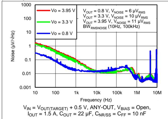
Figure 43. Spectral Noise Density vs Output Voltage
