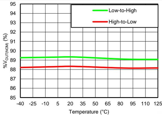
$V_{OUT(TARGET)} = 0.8\text{ V}$ ,  $V_{IN} = 6.5\text{ V}$ ,  $V_{BIAS} = \text{Open}$
