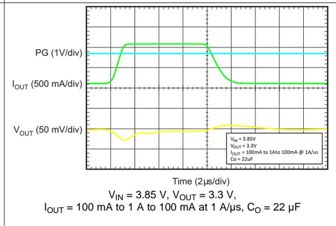
Figure 46. Load Transient Response
