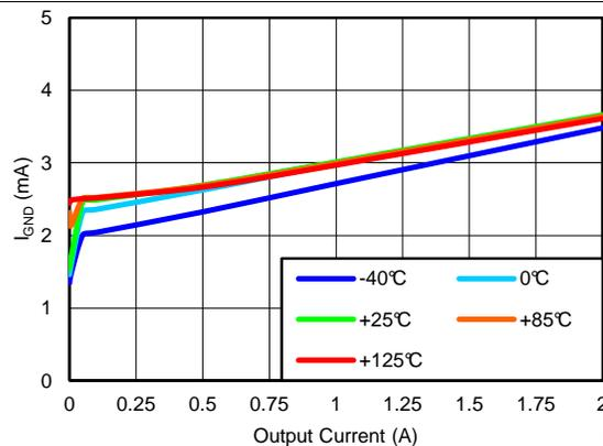
$V_{OUT(TARGET)} = 0.8\text{ V}$ ,  $V_{IN} = 1.4\text{ V}$ ,  $V_{BIAS} = \text{Open}$
