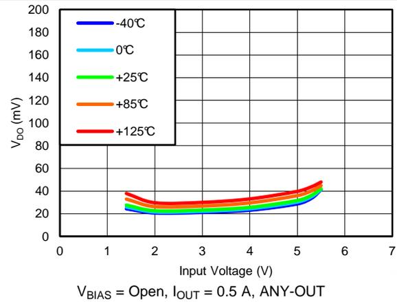
Figure 14. Dropout Voltage vs Input Voltage
