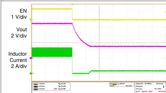
**Figure 9-6. Shutdown Waveforms**
