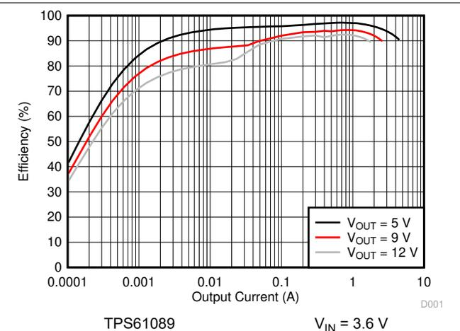
**Figure 7-2. Load Efficiency with Different Output Voltage**
