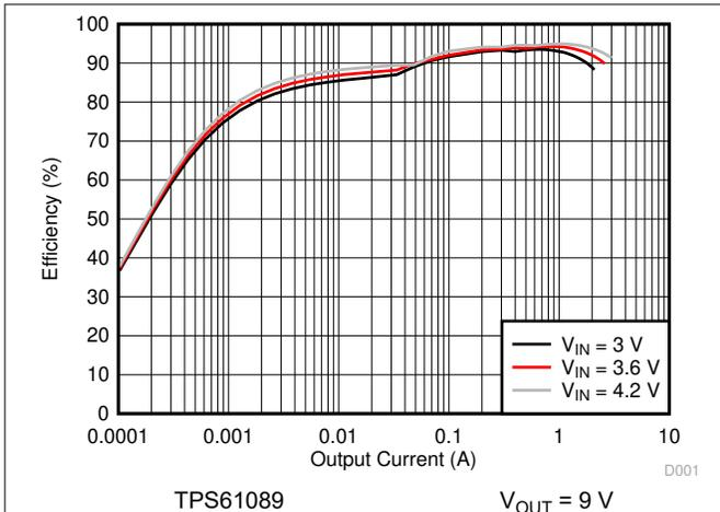
**Figure 7-1. Load Efficiency with Different Input Voltage**
