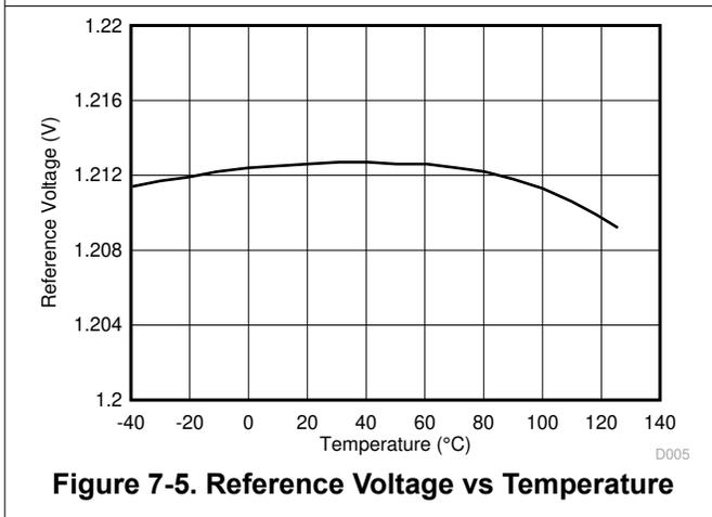
**Figure 7-5. Reference Voltage vs Temperature**
