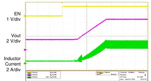
**Figure 9-5. Start-up Waveforms**
