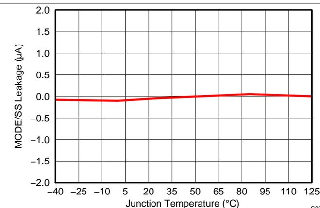
Figure 8. MODE/SS Leakage Current vs Junction Temperature
