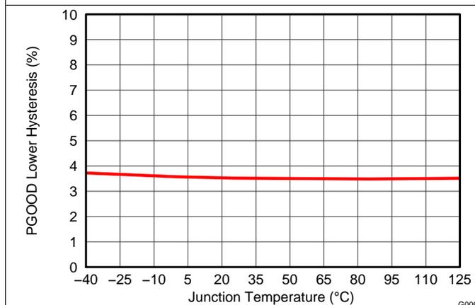
Figure 9. PGOOD Lower Hysteresis vs Junction Temperature
