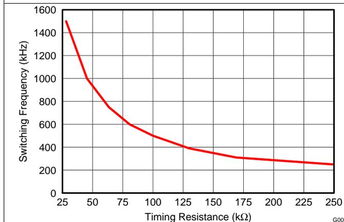
Figure 5. Switching Frequency vs Timing Resistance ( $R_T$ )
