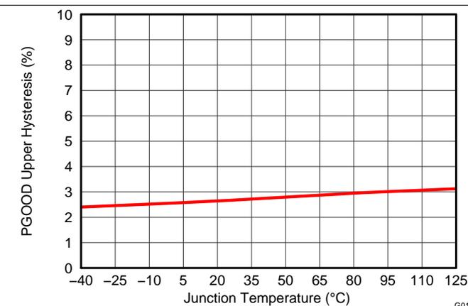
Figure 10. PGOOD Upper Hysteresis vs Junction Temperature
