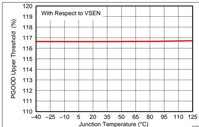
Figure 7. PGOOD Upper Threshold vs Junction Temperature
