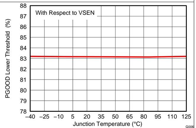
Figure 6. PGOOD Lower Threshold vs Junction Temperature
