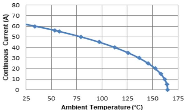
**Figure 5: Maximum Continuous Current at a Given  $T_A$**
