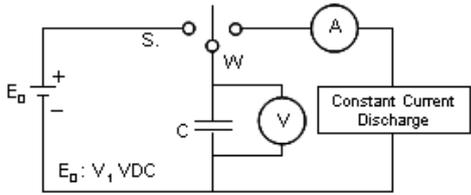
$C = A(\text{Ampere}) \times T \text{ sec} / (V_1 - V_2) \text{ V [F]}$
