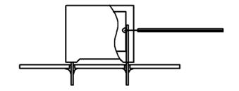
Temperature monitored inside the capacitor.
