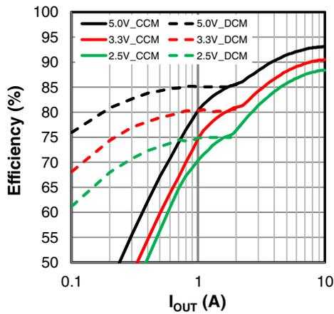
Figure 17: Efficiency, V<sub>IN</sub>=24V, f=500kHz
