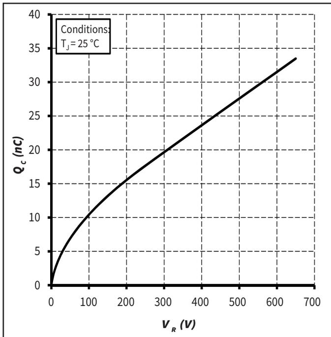
Figure 5. Total Capacitance Charge vs. Reverse Voltage
