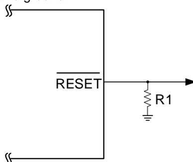
**Figure 1.  $\overline{RESET}$  Valid to Ground Circuit**
