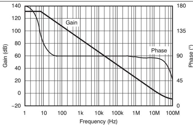
Figure 9. Open-Loop Gain and Phase vs Frequency
