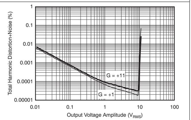
Figure 4. Total Harmonic Distortion + Noise Ratio vs Amplitude
