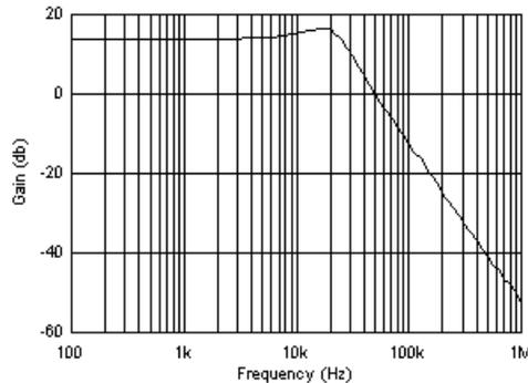
**Figure 36. OPAx209 Second-Order, 25-kHz, Chebyshev, Low-Pass Filter**
