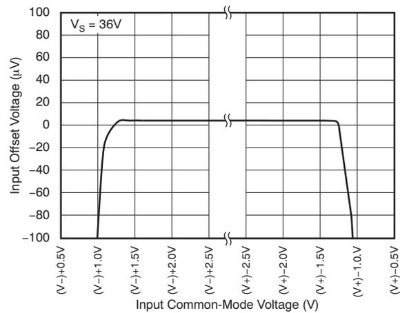
**Figure 14. Input Offset Voltage vs Common-Mode Voltage**
