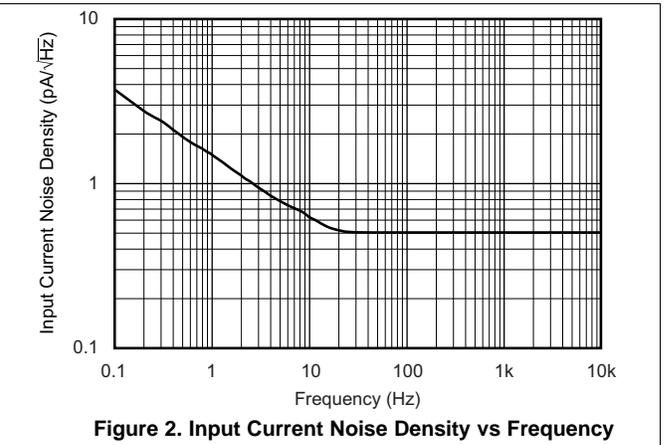
Figure 2. Input Current Noise Density vs Frequency
