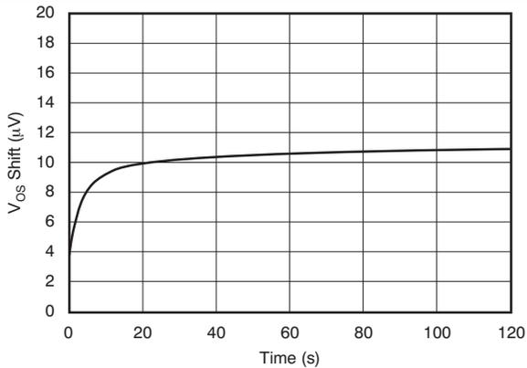
**Figure 15. Input Offset Voltage vs Time**
