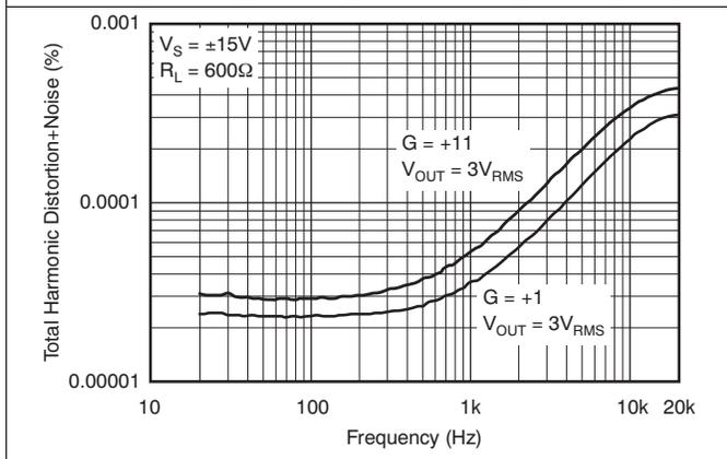
Figure 3. Total Harmonic Distortion + Noise Ratio vs Frequency
