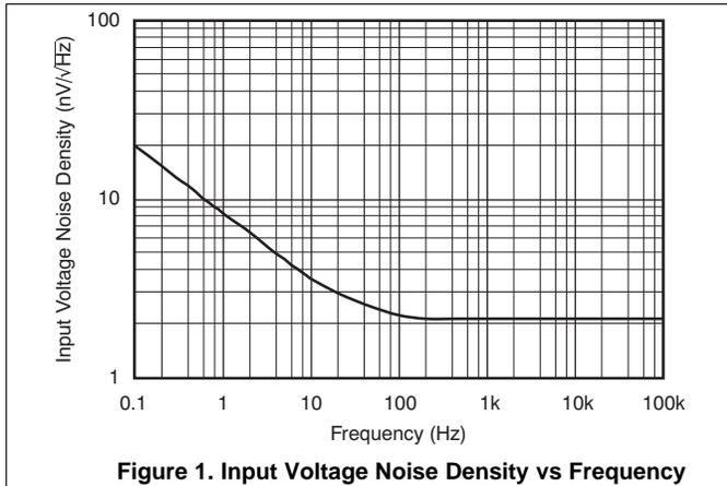
Figure 1. Input Voltage Noise Density vs Frequency
