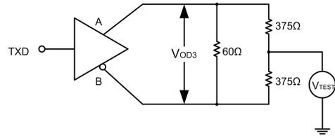
Figure 10. Driver Test Circuit, VOD With Common-Mode Loading
