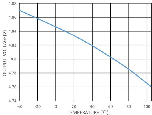
Figure5. Receiver Output High Voltage vs. Temperature
