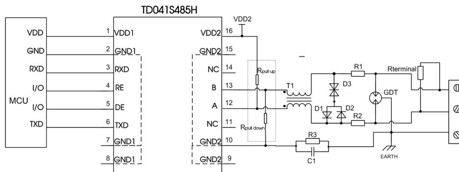
Figure 14. Port protection circuit for harsh environments
