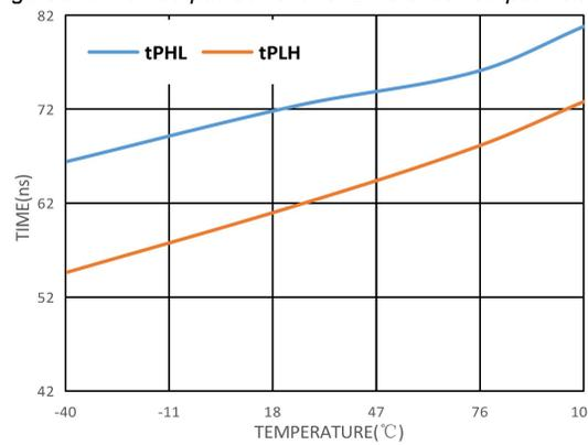
Figure 8. Receiver Propagation Delay vs. Temperature
