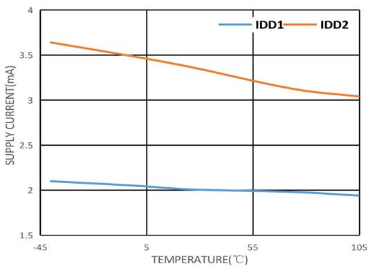
Figure3. Unloaded Supply Current vs. Temperature
