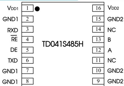
Note: All GND1 pins are internally connected;
