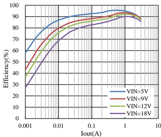
**Figure 3. Efficiency vs. Load Current,  $V_{OUT} = 3.3V$**
