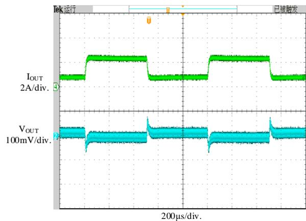
**Figure 12. Load Transient,
