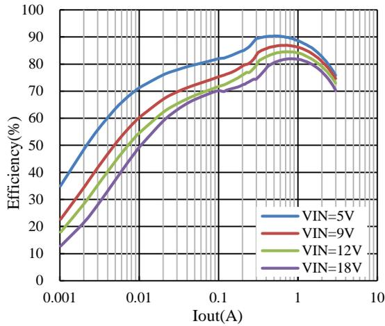
**Figure 1. Efficiency vs. Load Current,  $V_{OUT} = 1.2V$**
