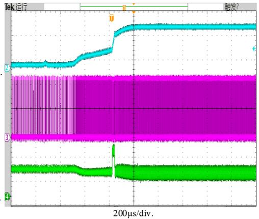
**Figure 10. Short Circuit Recovery**
