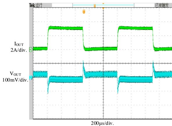
**Figure 11. Load Transient,
