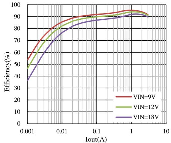
**Figure 4. Efficiency vs. Load Current,  $V_{OUT} = 5V$**
