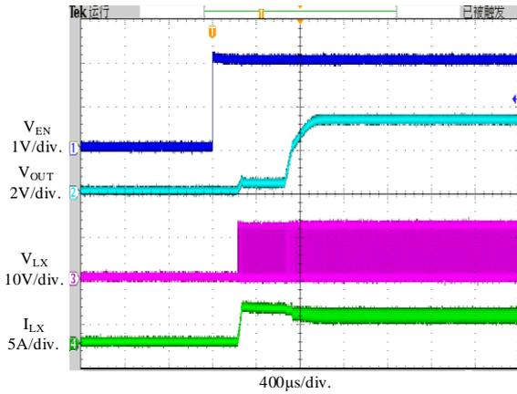
**Figure 7. Startup Waveforms**
