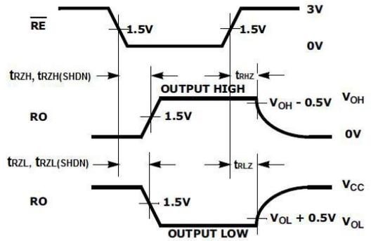
Figure 8 : Receiver Enable and Disable Times
