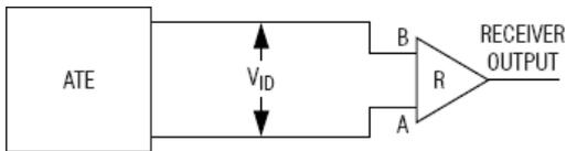
Figure 9 : Receiver Propagation Delay Test Circuit
