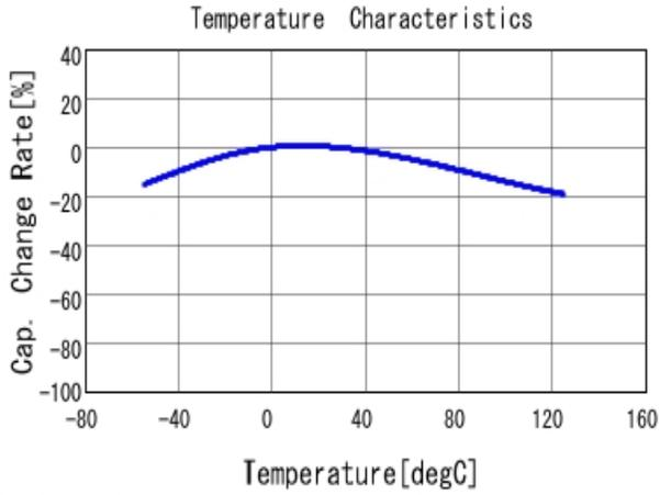
■ GRM155C71A225KE11 C-Temp. capchange, DCO. 0V, ACO. 1V<sub>rm</sub>
