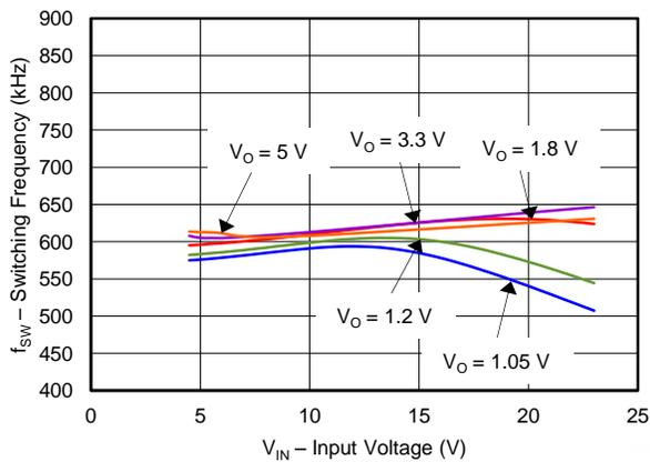
**Figure 9. SWITCHING FREQUENCY vs INPUT VOLTAGE (I<sub>0</sub> = 1 A)**
