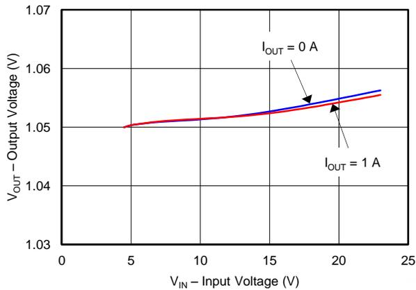
Figure 5. 1.05-V OUTPUT VOLTAGE vs INPUT VOLTAGE
