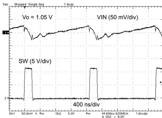
**Figure 13. VOLTAGE RIPPLE AT INPUT (IO = 3 A)**
