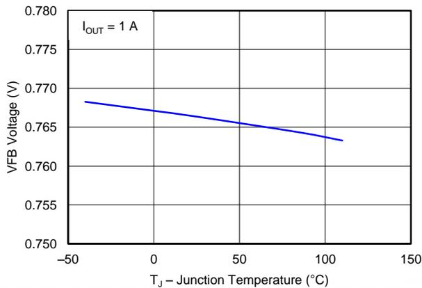
**Figure 11. VFB VOLTAGE vs JUNCTION TEMPERATURE (I<sub>0</sub> = 1 A)**
