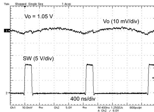
**Figure 12. VOLTAGE RIPPLE AT OUTPUT (I<sub>0</sub> = 3A)**
