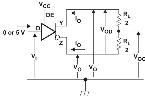
Figure 1. Driver  $V_{OD}$  Test Circuit and Current Definitions
