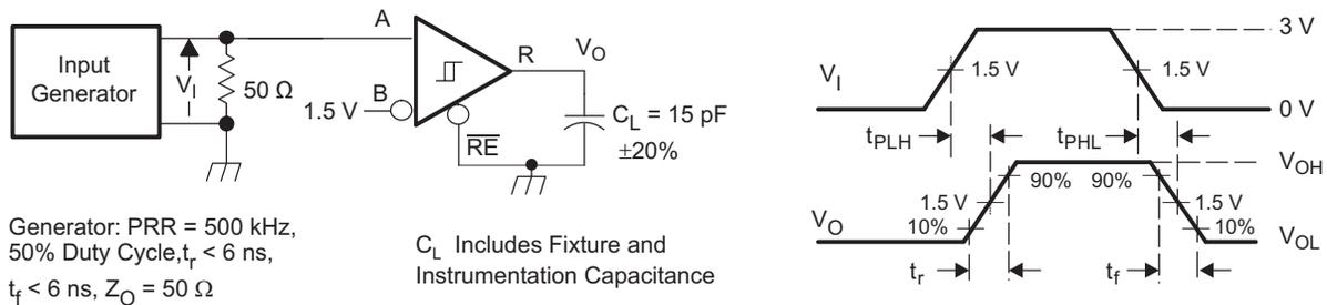
Figure 8. Receiver Switching Test Circuit and Voltage Waveforms
