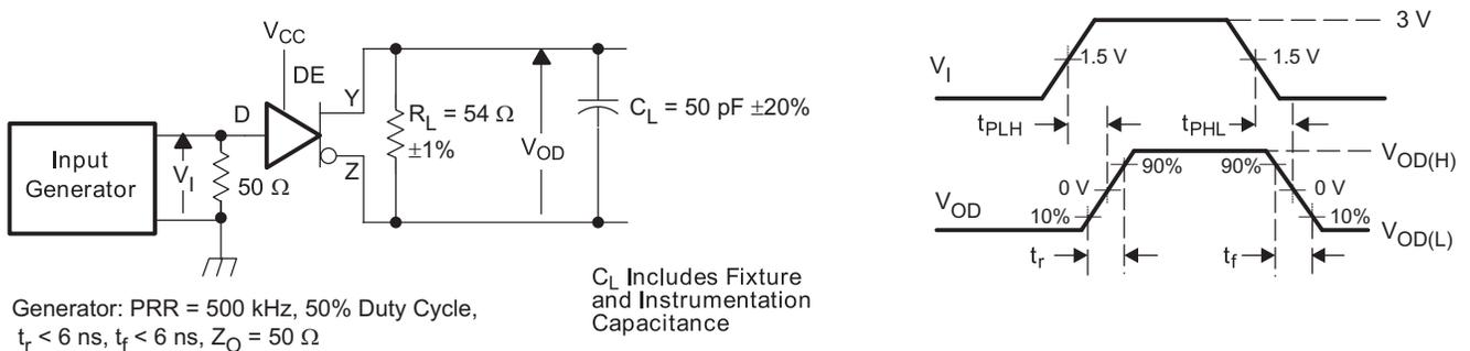
Figure 4. Driver Switching Test Circuit and Voltage Waveforms
