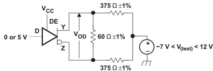
Figure 2. Driver  $V_{OD}$  With Common-Mode Loading Test Circuit
