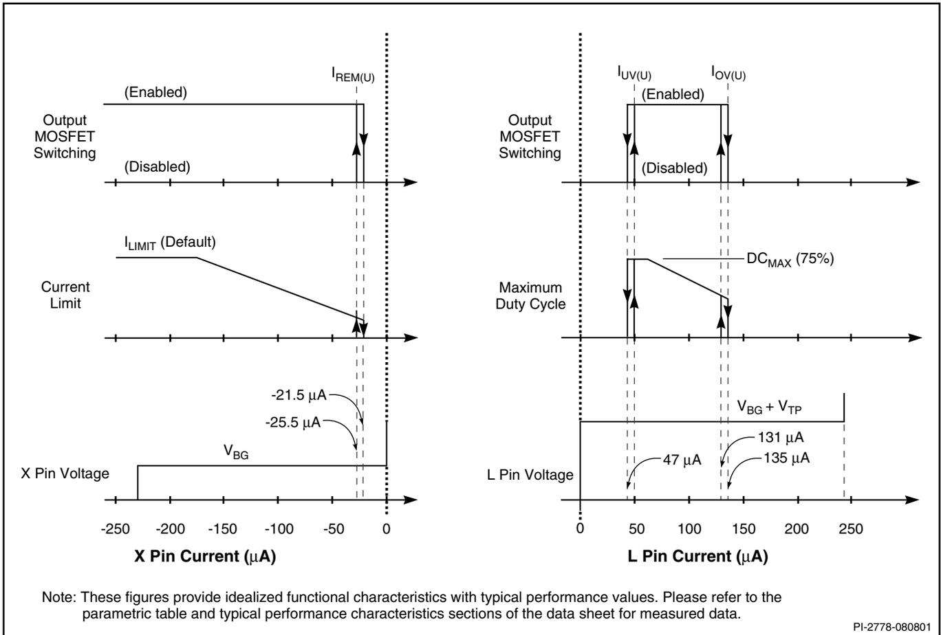
Figure 7. LINE-SENSE and EXTERNAL CURRENT LIMIT Pin Characteristics.
