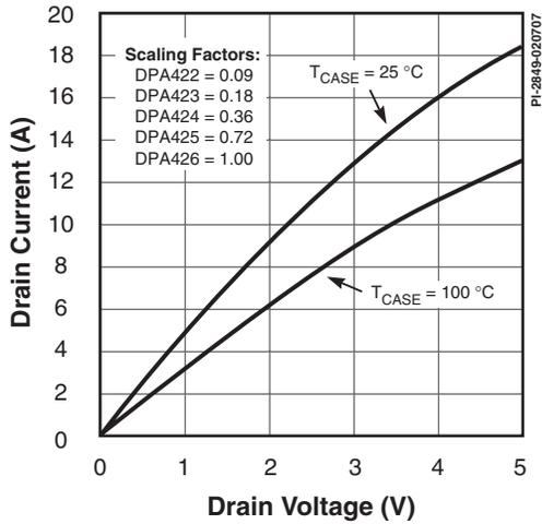
Figure 48. Output Characteristics.
