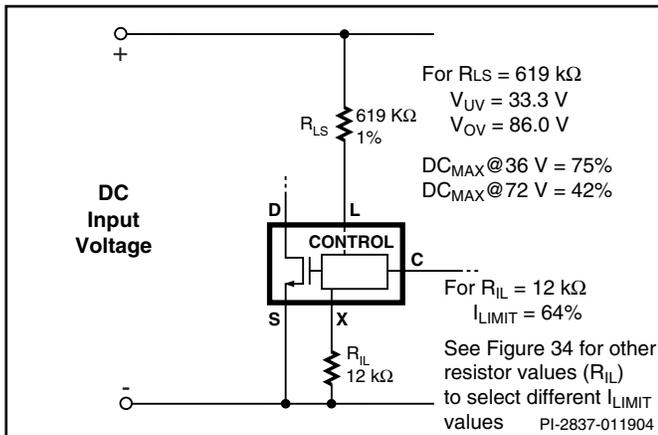
Figure 23. Line-Sensing and Externally Set Current Limit.
