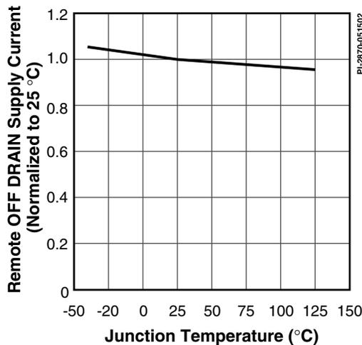
Figure 46. Remote OFF DRAIN Supply Current vs. Temperature.
