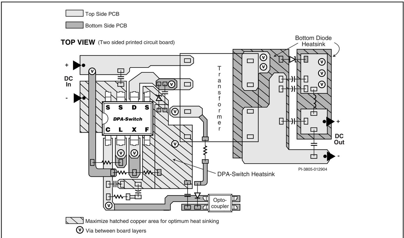
Figure 29. Layout Considerations for DPA-Switch Using G Package.
