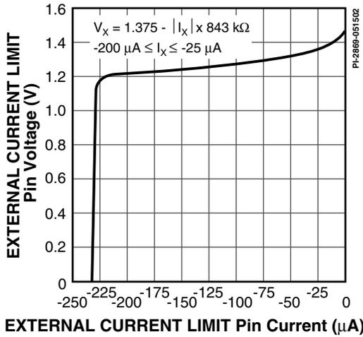
Figure 42. EXTERNAL CURRENT LIMIT Pin Voltage vs. Current
